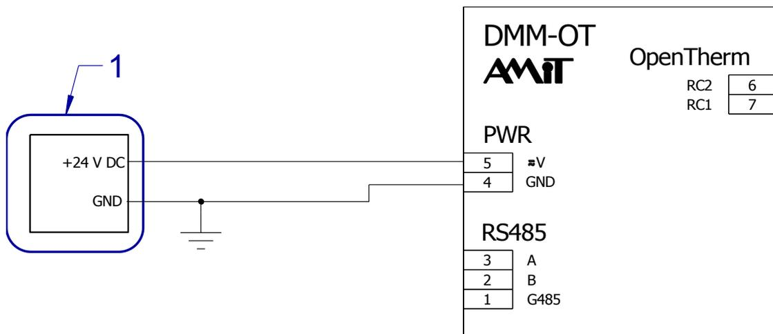
Fig. 4 - Example of DC power supply connection
