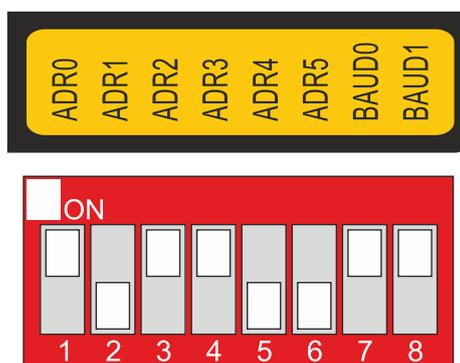
Fig. 11 - DIP switch for setting the communication parameters
