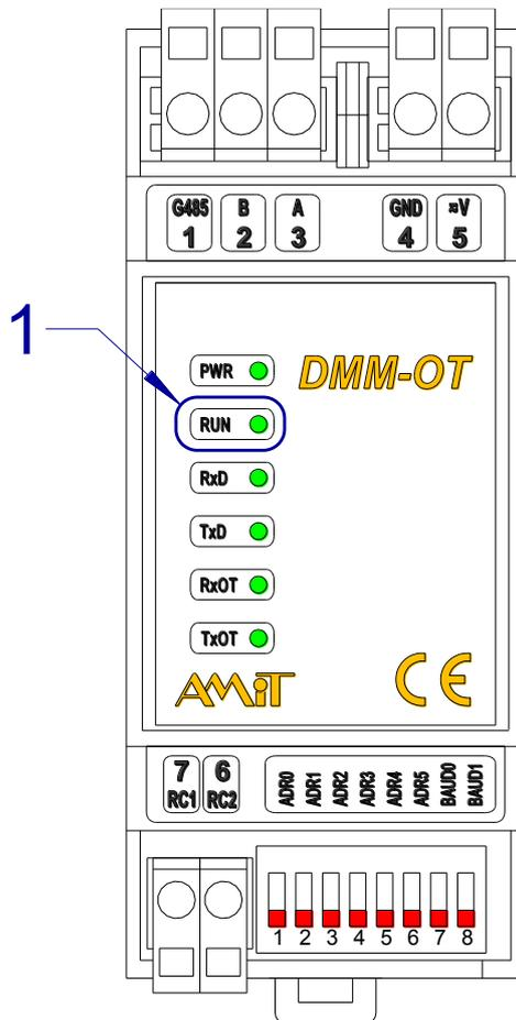
Fig. 10 - RUN indication LED location
