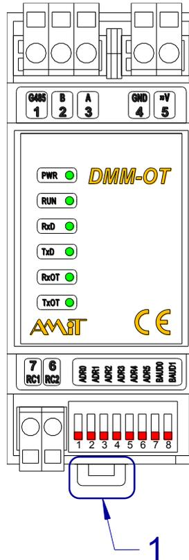
Fig. 12 - Position of locking latch for DIN rail
