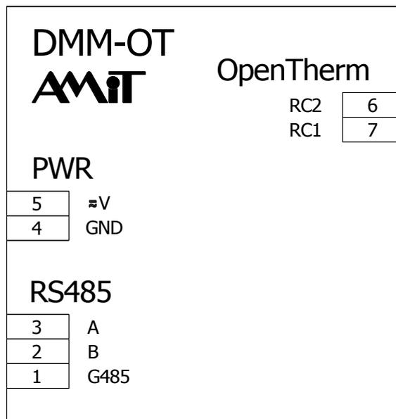
Fig. 2 - Recommended drawing symbol for **DMM-OT**
