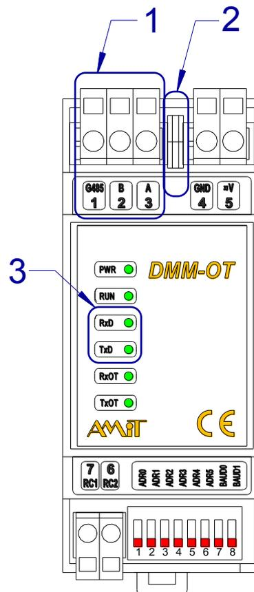
Fig. 6 - Location of connector, configuration jumpers and indication LEDs
