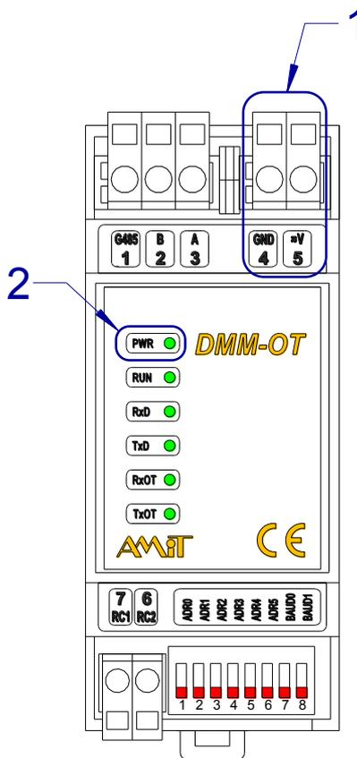
Fig. 3 - Power supply connector and LED indicator location
