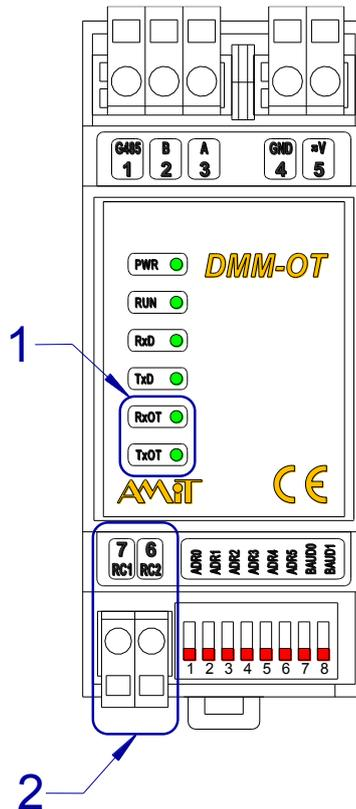
Fig. 9 - Location of connectors and indication LEDs
