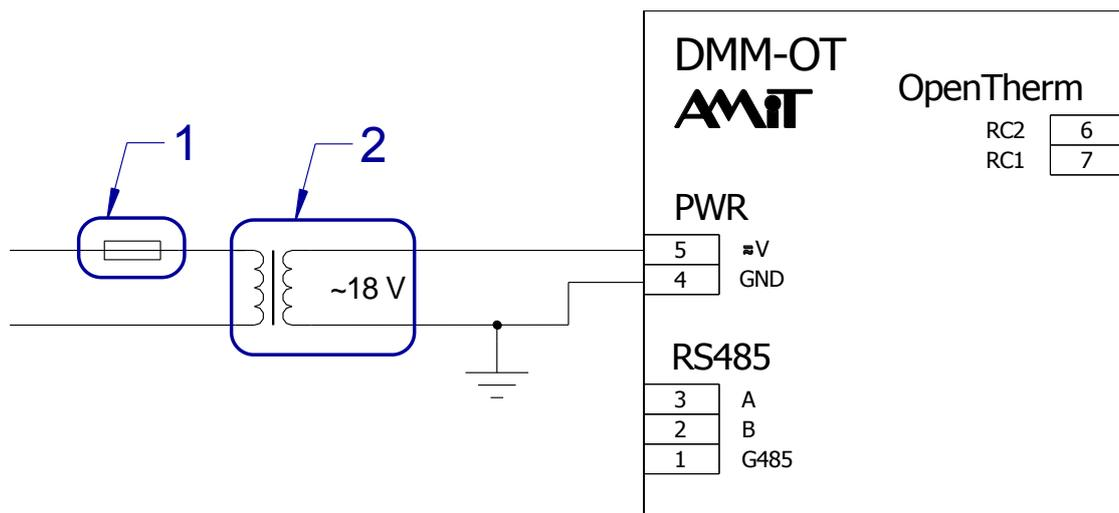
Fig. 5 - Example of AC power supply connection
