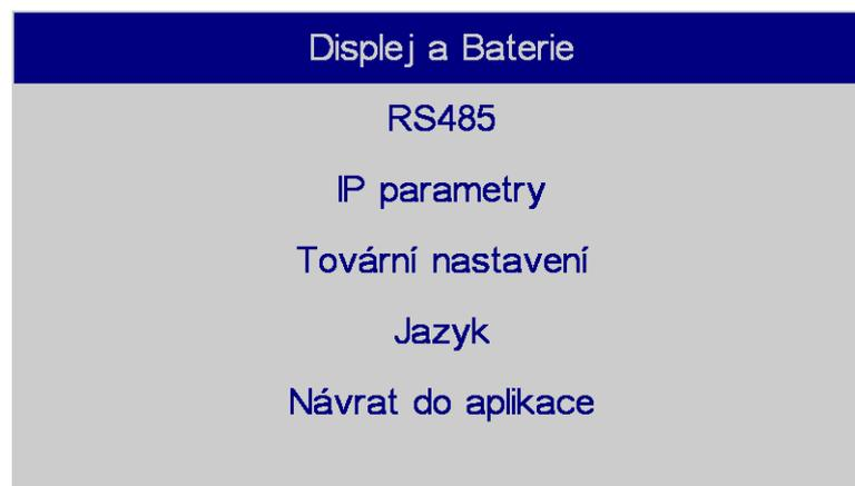
Fig. 13 - Service mode menu, called-out by touching the screen
