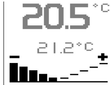
Fig. 13 – Correction of required temperature
