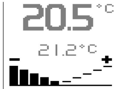
Fig. 13 - Correction of required temperature
