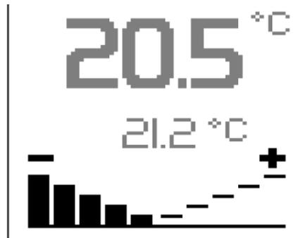
Fig. 15 - Correction of requested temperature
