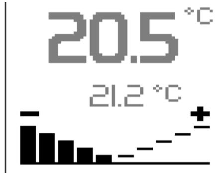
Fig. 16 - Correction of required temperature
