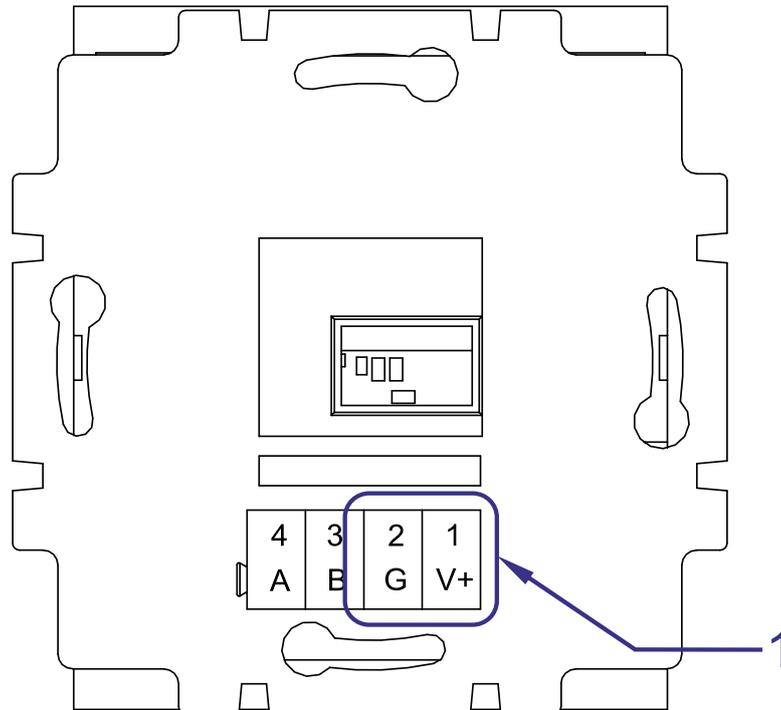
Fig. 3 - Location of power supply connector
