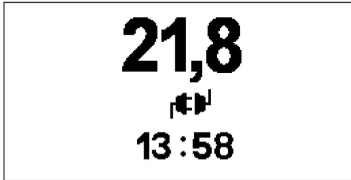
Fig. 40 - Communication interruption during active screen saver
