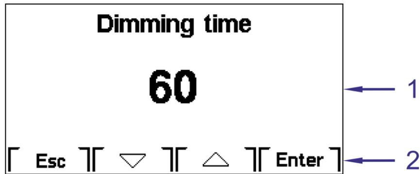
Fig. 26 - Setting time for screen saver activation
