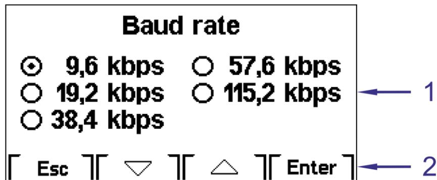
Fig. 35 - Setting communication speed
