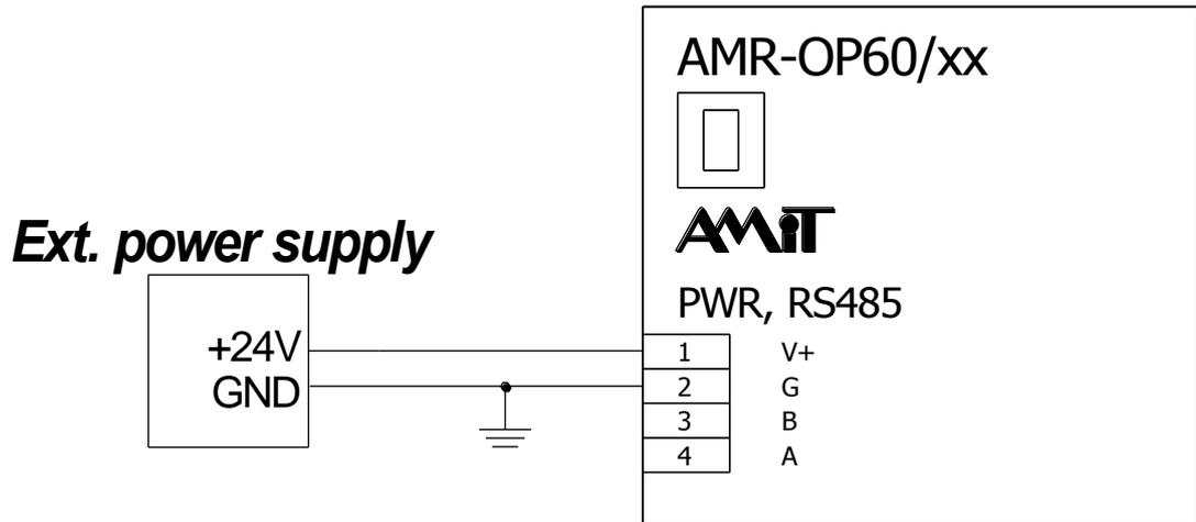
Fig. 4 - Power supply wiring example
