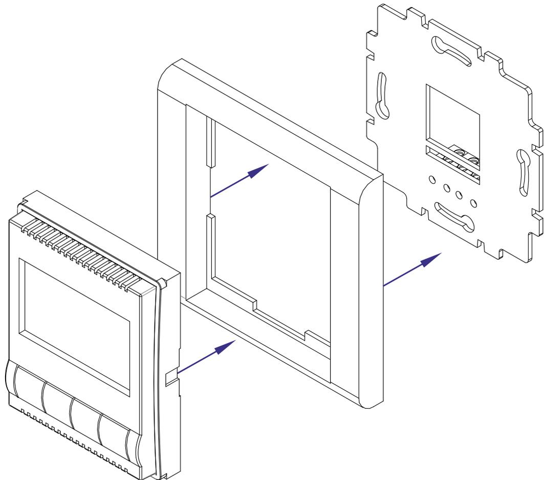
Fig. 10 - On-wall controller installation
