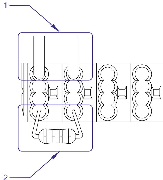
Fig. 9 - Connecting to connection points (poles detail in plan view)
