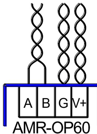
Fig. 7 - Connecting structured cabling to poles of controller
