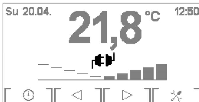
Fig. 39 - Communication interruption on basic screen
