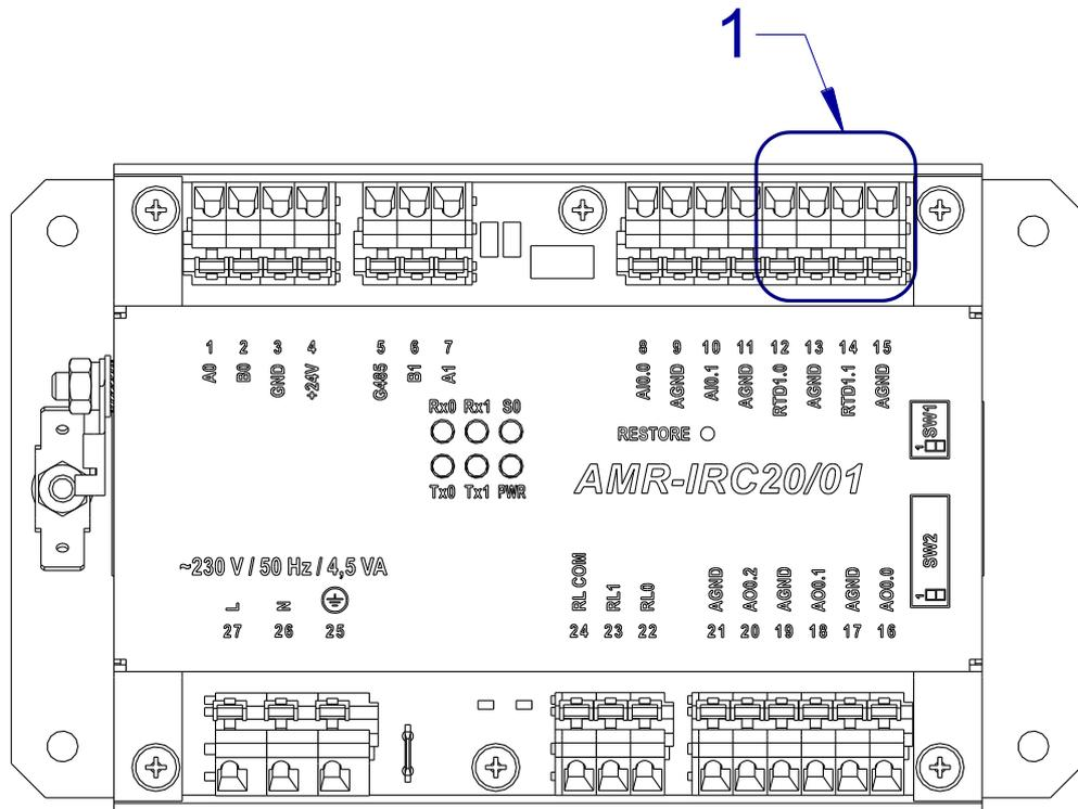
Fig. 12 – Terminals location for RTD inputs
