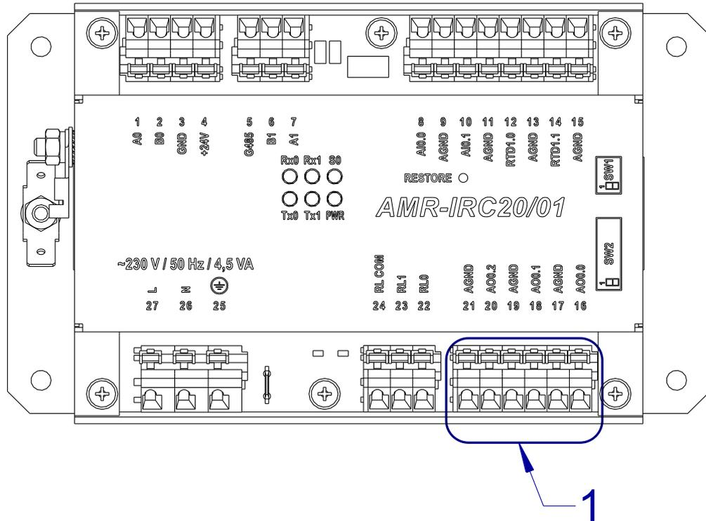
Fig. 15 – Terminals location for analogue outputs
