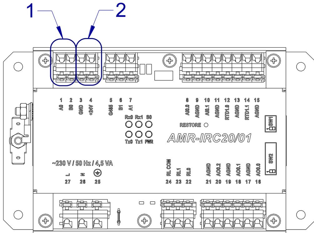
Fig. 6 – Terminals location for on-wall controller connection
