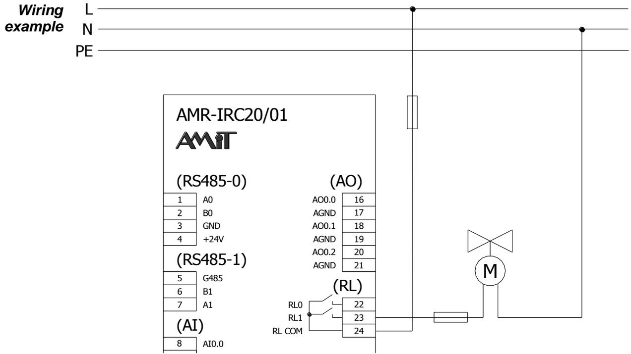
Fig. 18 – Wiring example of thermoelectric head connection to relay output
