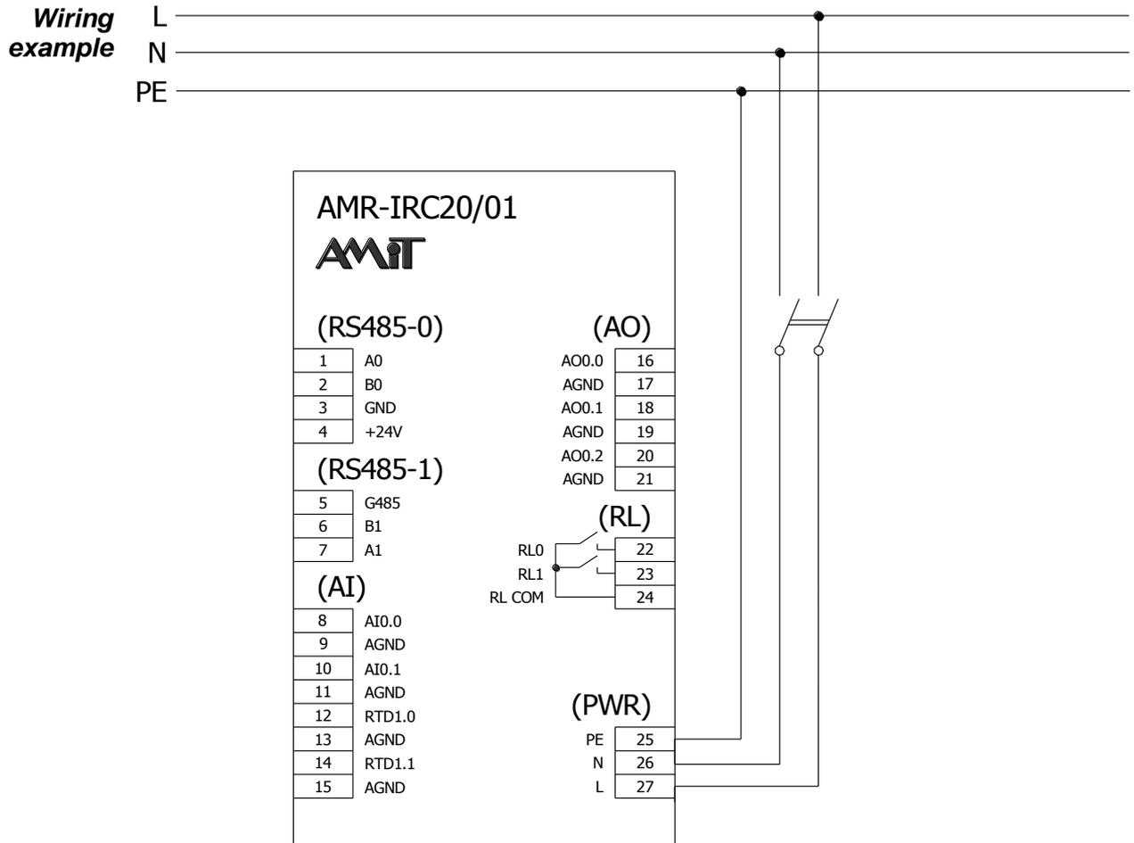
Fig. 4 – Power supply wiring example
