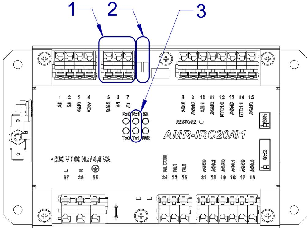
Fig. 9 – Terminals and LEDs location for RS485 with GI
