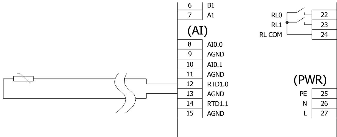
Fig. 13 – Temperature sensor wiring example
