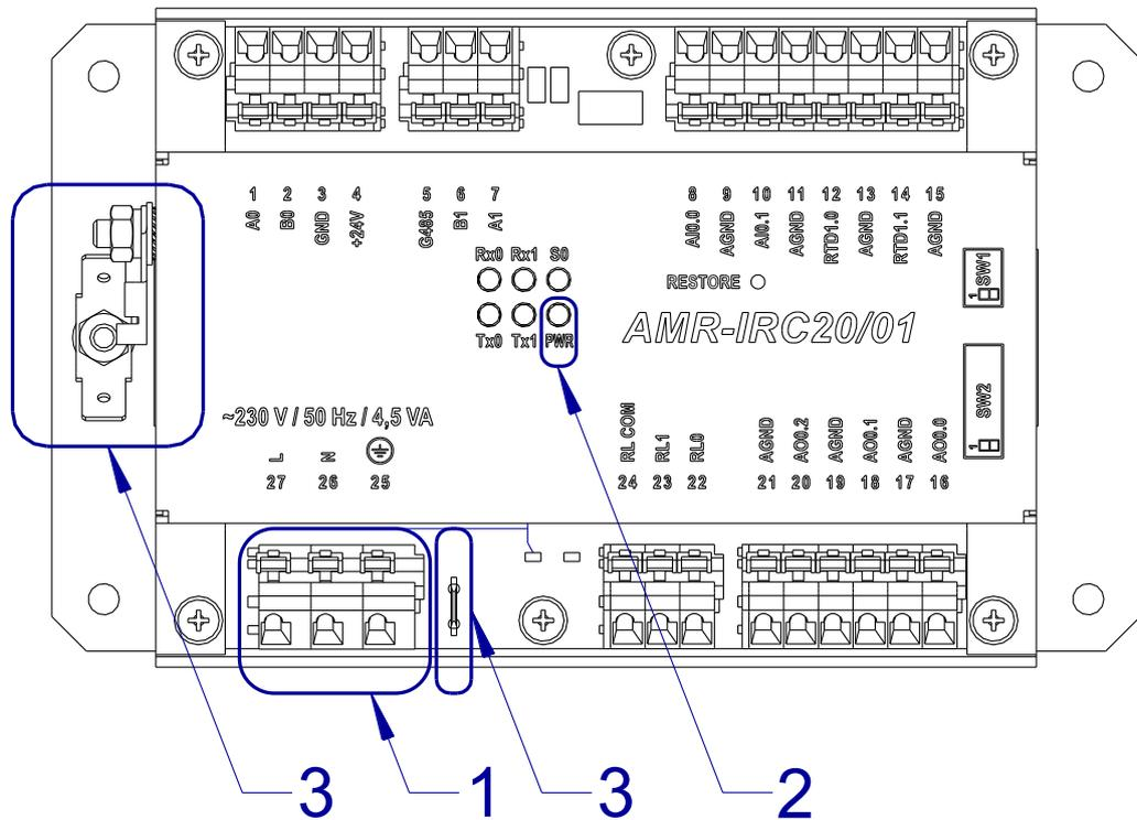
Fig. 3 – Terminals location for power supply
