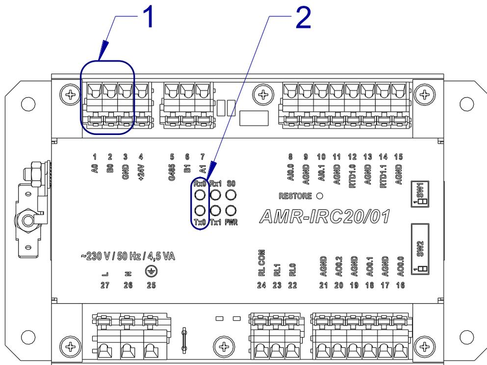
Fig. 5 – Terminals and LEDs location for RS485 without GI
