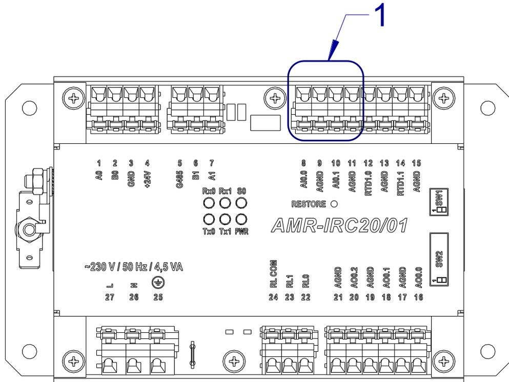
Fig. 10 – Terminals for analogue input
