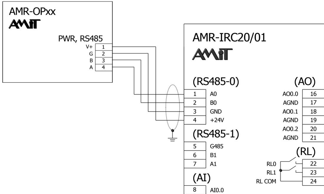
Fig. 7 – Wiring example of on-wall controller connection to **AMR-IRC20/01**
