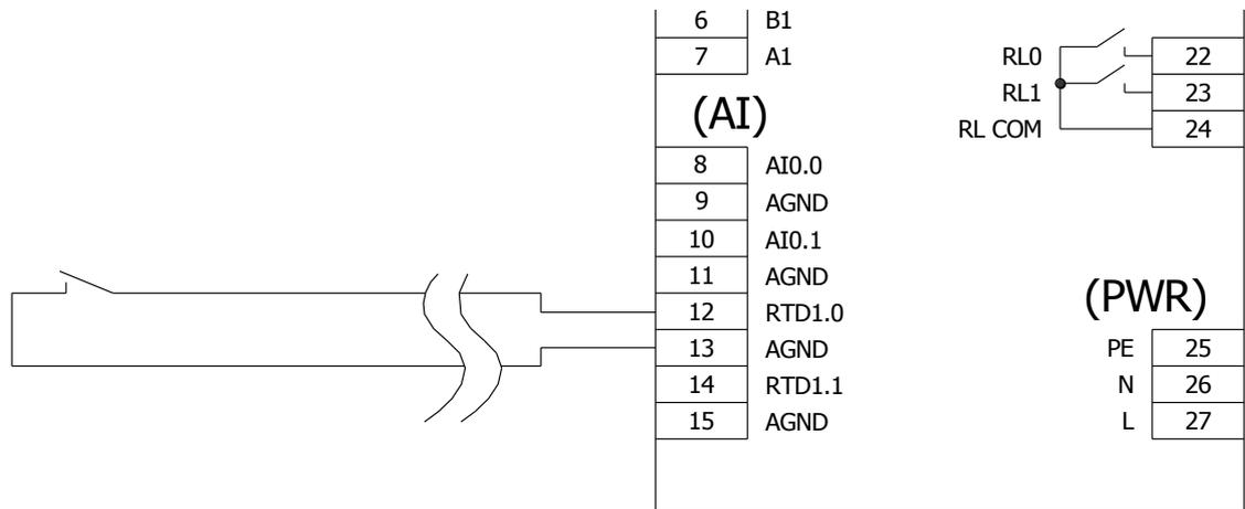
Fig. 14 – Dry contact wiring example
