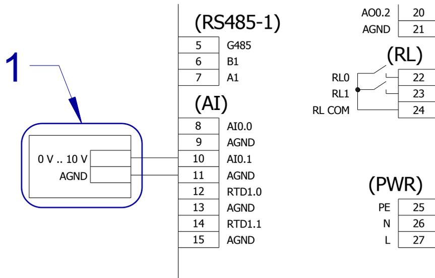
Fig. 11 – Voltage sensor 0 V to 10 V connection
