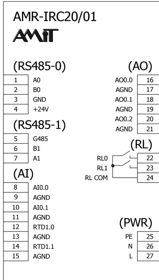
Fig. 2 – Recommended drawing symbol for **AMR-IRC20/01**
