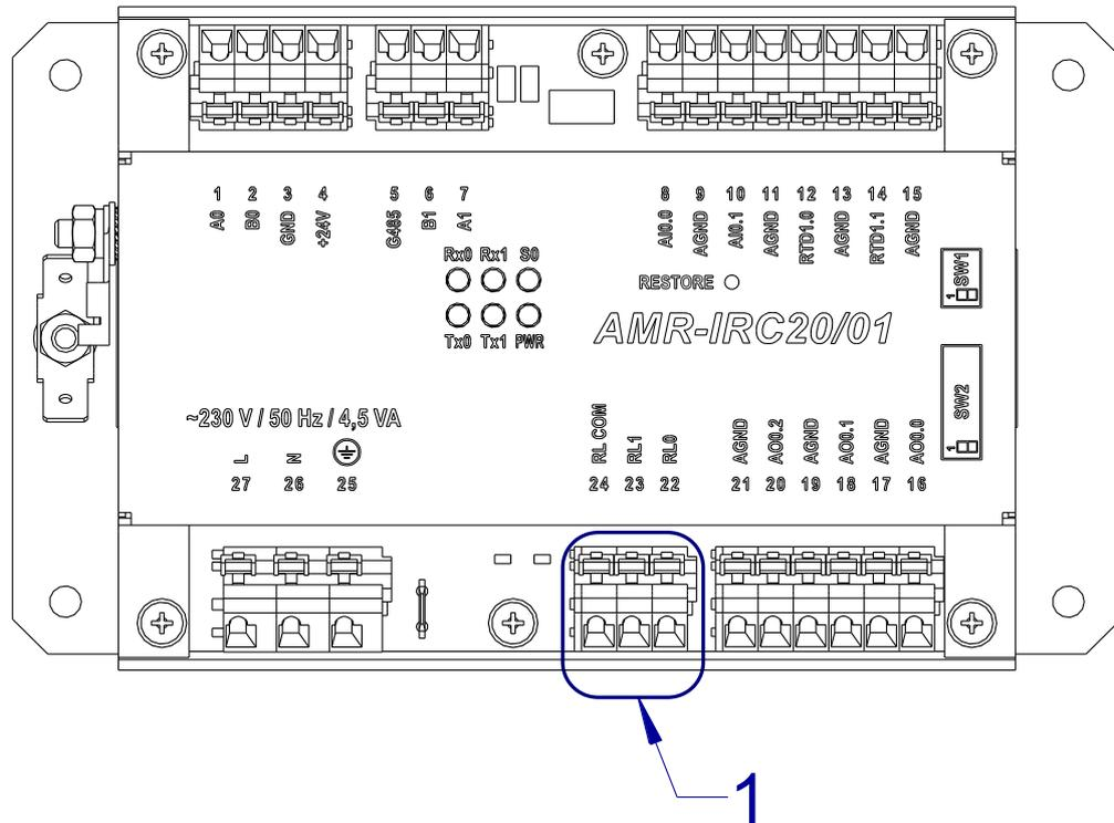
Fig. 17 – Terminals location for relay outputs
