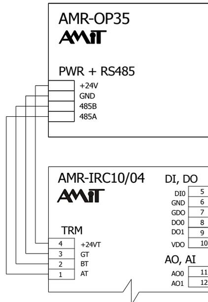
Fig. 17 – Wiring example of the room controller **AMR-OP35**
