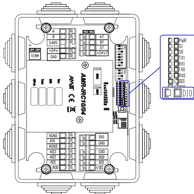
Fig. 10 – Digital input status LEDs
