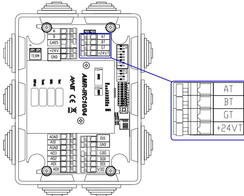
Fig. 15 – RS485 interface terminals location
