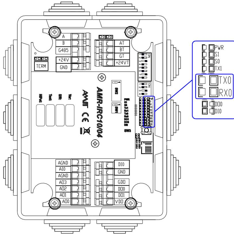
Fig. 16 – Location of RS485 interface status LEDs for room controller
