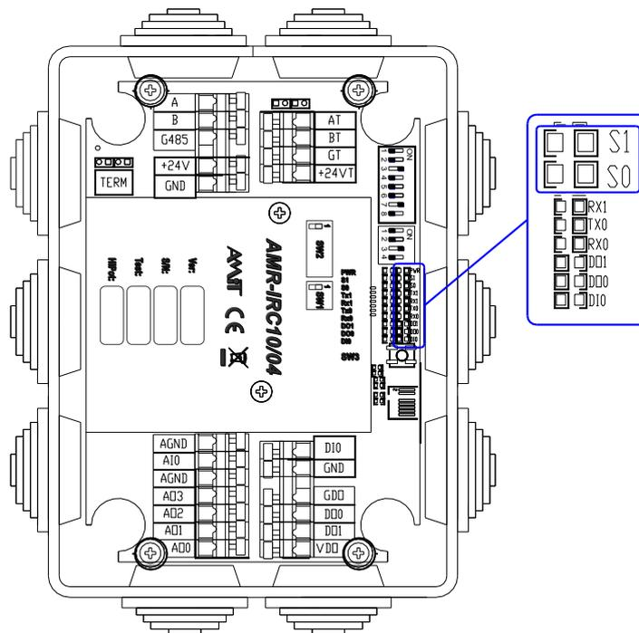
Fig. 25 – Service LEDs location
