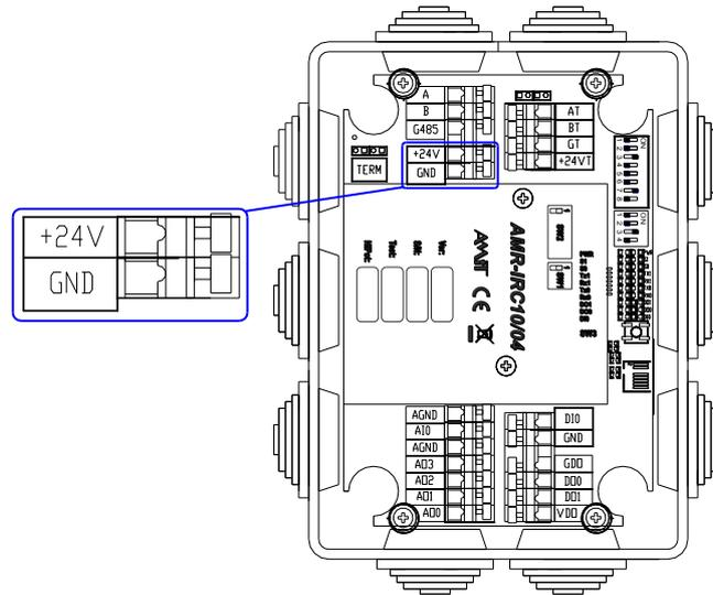
Fig. 3 – Power supply terminals location
