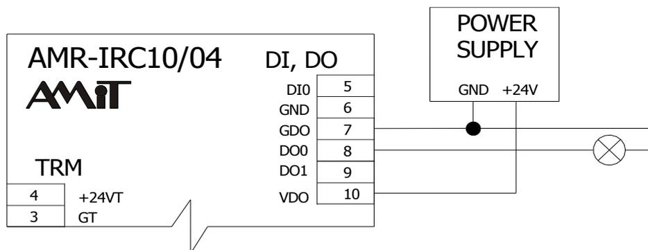
Fig. 14 – Signal light wiring to DO0 output
