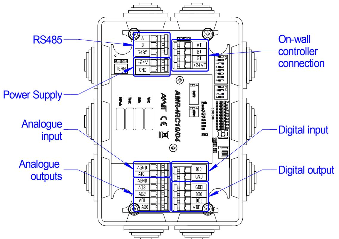
Fig. 21 – Connector location
