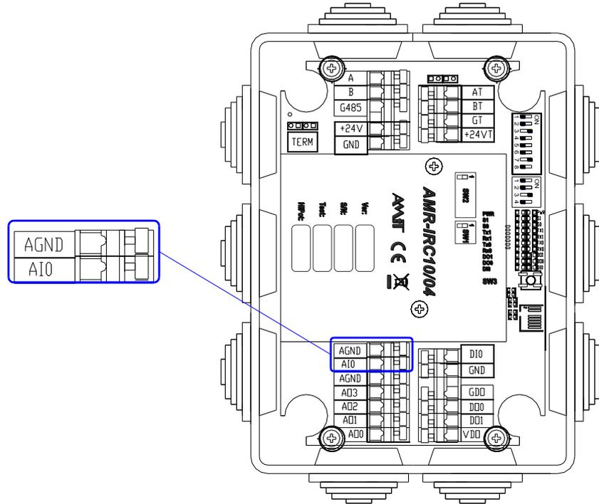
Fig. 5 – Analogue input terminals location
