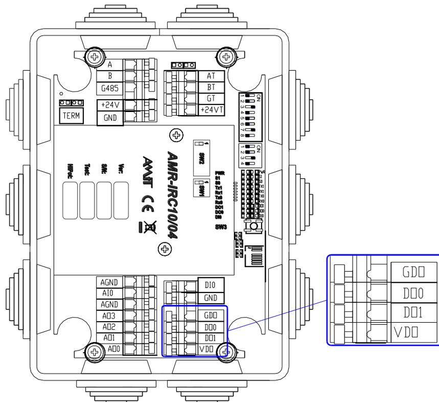
Fig. 12 – Digital output terminals location
