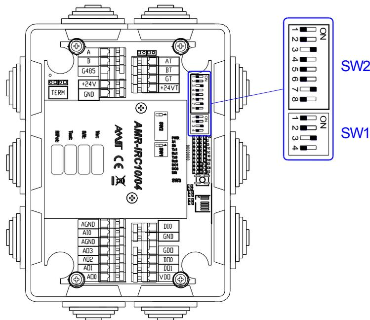
Fig. 24 – Configuration DIP switches location
