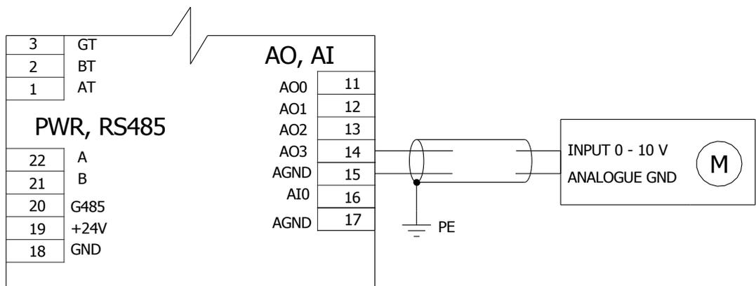
Fig. 8 – Example of wiring a drive to AO3 analogue output
