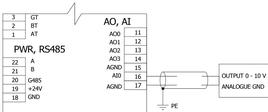
Fig. 6 – AI wiring example
