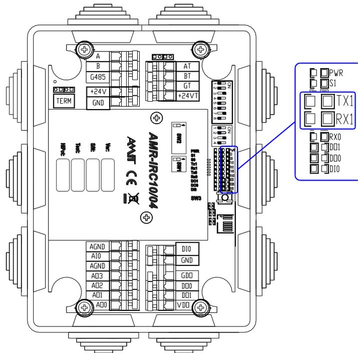
Fig. 19 – Status LEDs of RS485 interface without GI
