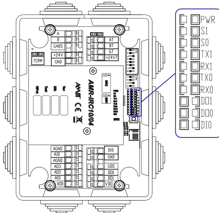
Fig. 22 – Status LEDs location
