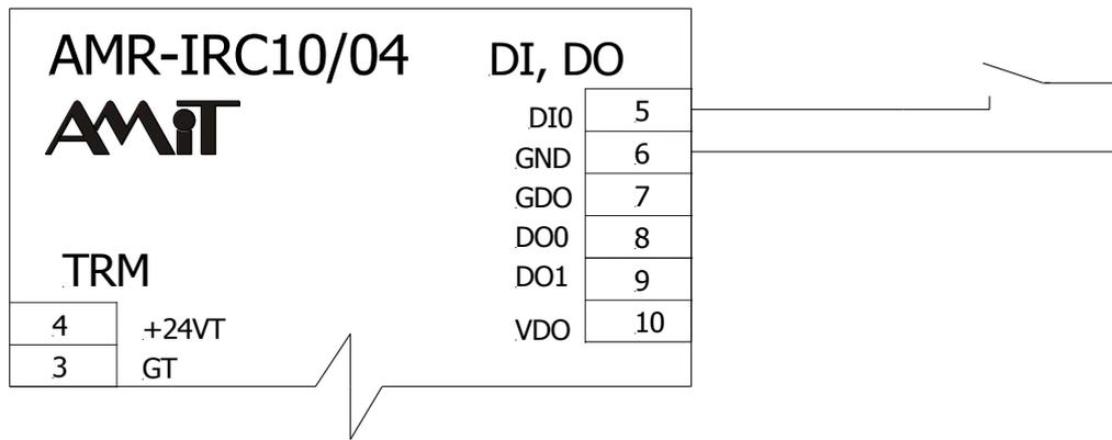
Fig. 11 – Example of contact wiring to DI0
