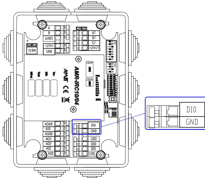
Fig. 9 – Digital input terminals location
