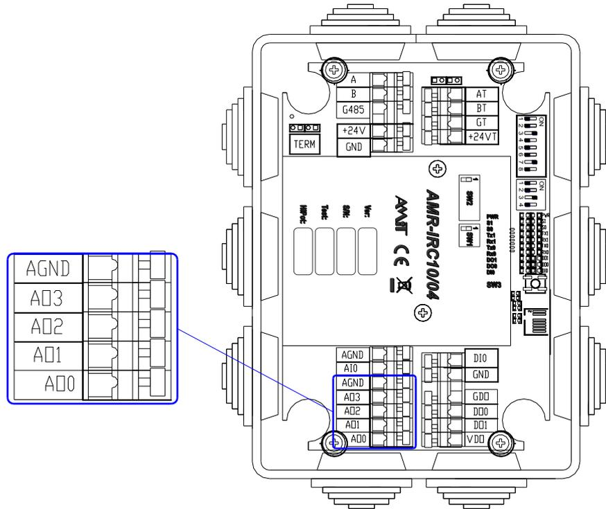
Fig. 7 – Analogue output terminals location
