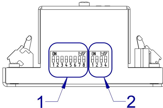
Fig. 18 – DIP switch location for communication parameters setting
