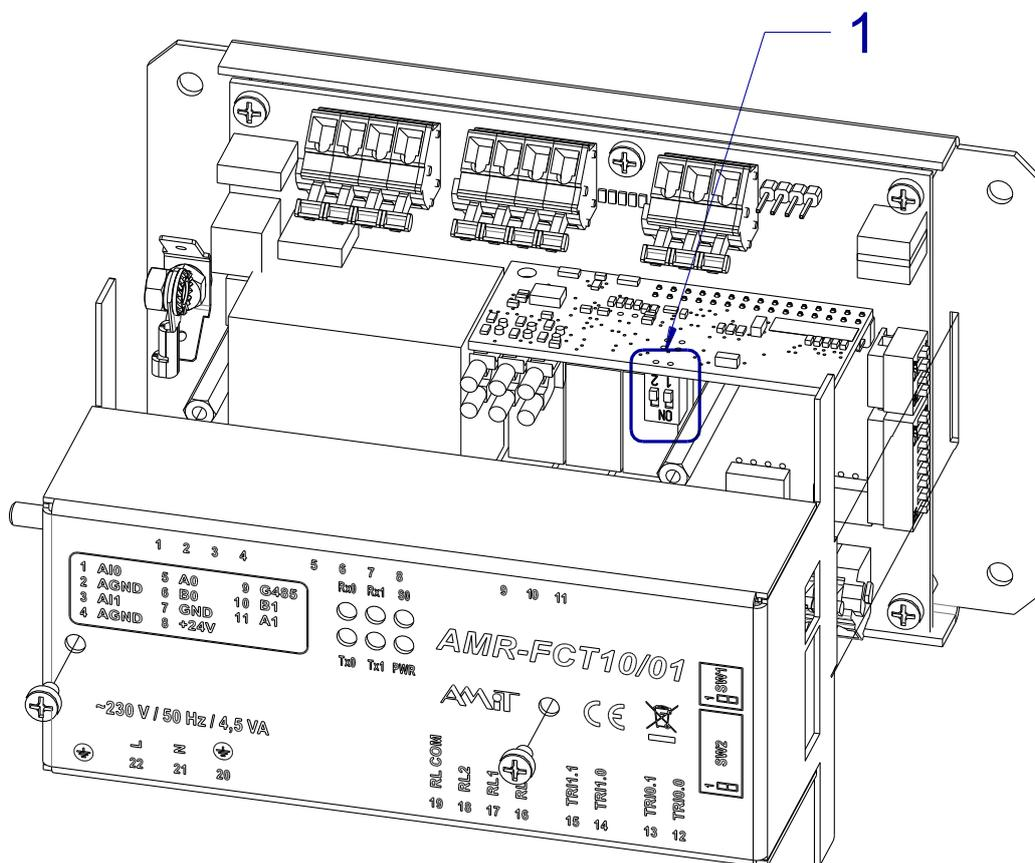
Fig. 20 – Service DIP switch location
