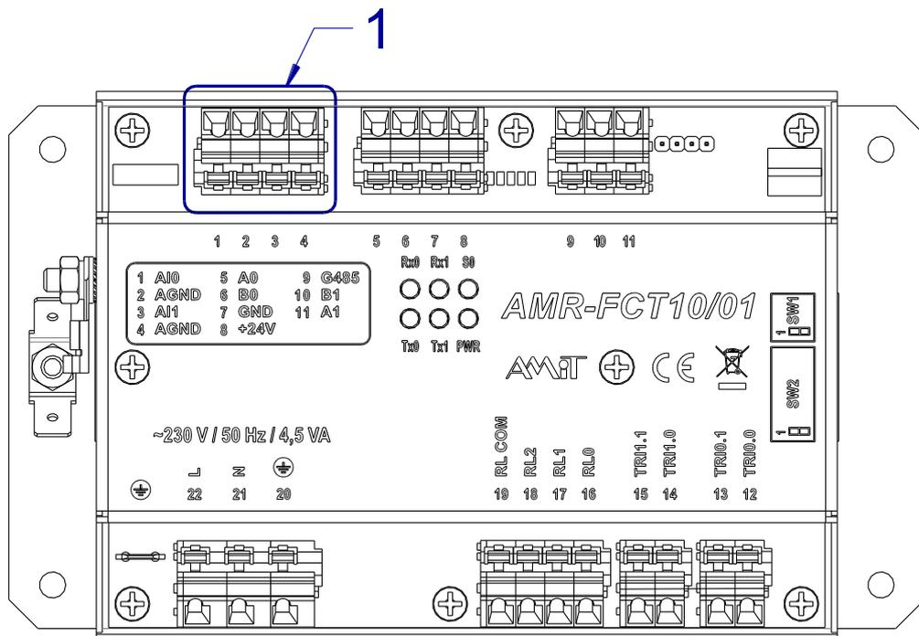
Fig. 10 – Location of terminals for RTD inputs
