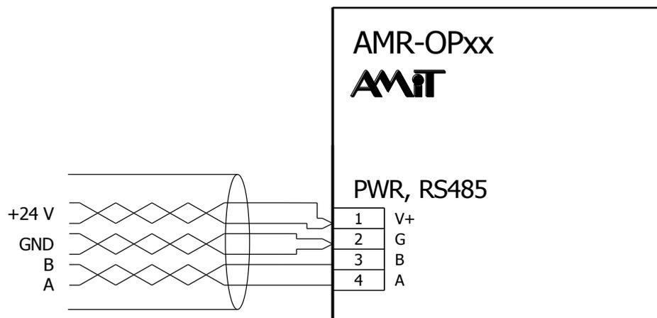
Fig. 8 – Structured cabling use example
