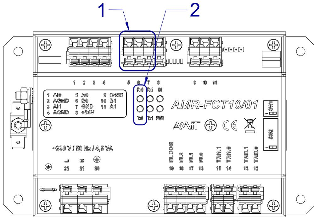
Fig. 5 – Terminals and LEDs location for RS485 without GI
