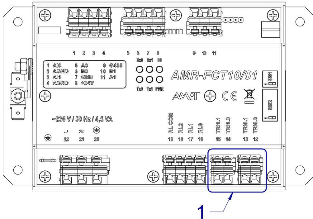
Fig. 15 – Location of triac outputs terminals
