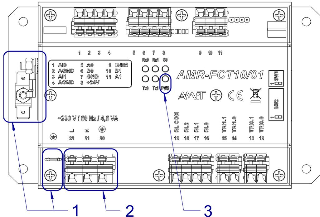
Fig. 3 – Terminals location for power supply
