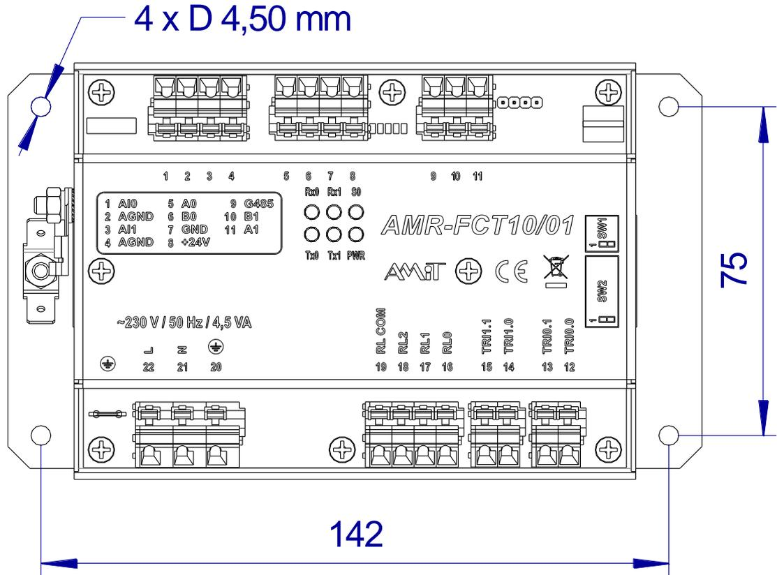
Fig. 17 – Dimensions of mounting holes
