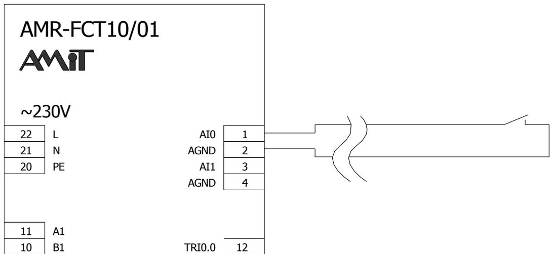
Fig. 12 – Dry contact wiring example
