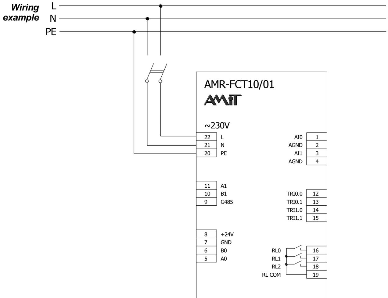
Fig. 4 – Power supply wiring example
