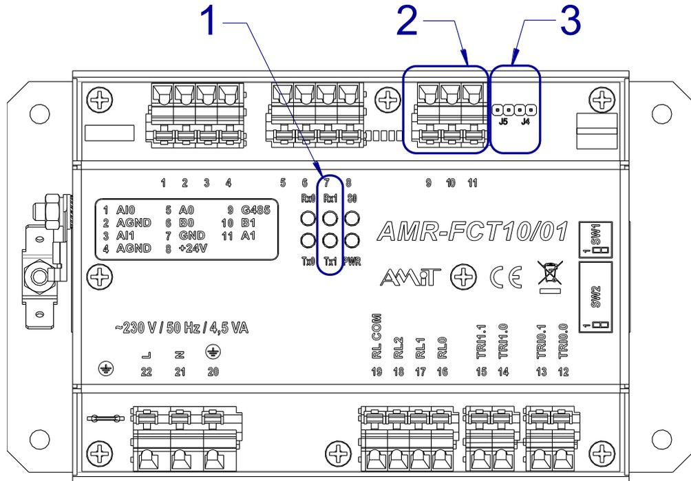
Fig. 9 – Terminals and LEDs location for RS485 with GI
