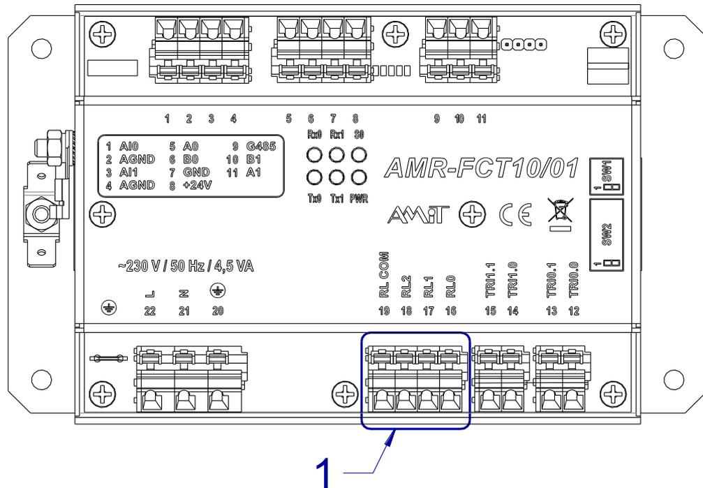
Fig. 13 – Terminals location for relay outputs
