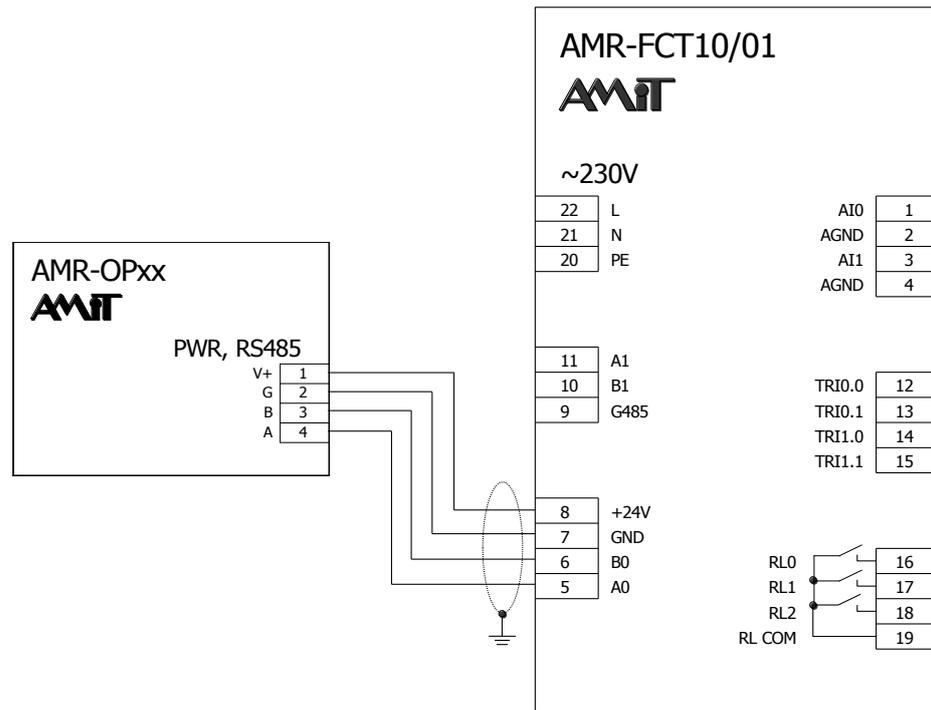
Fig. 7 – Wiring example of on-wall controller connection to **AMR-FCT10/01**
