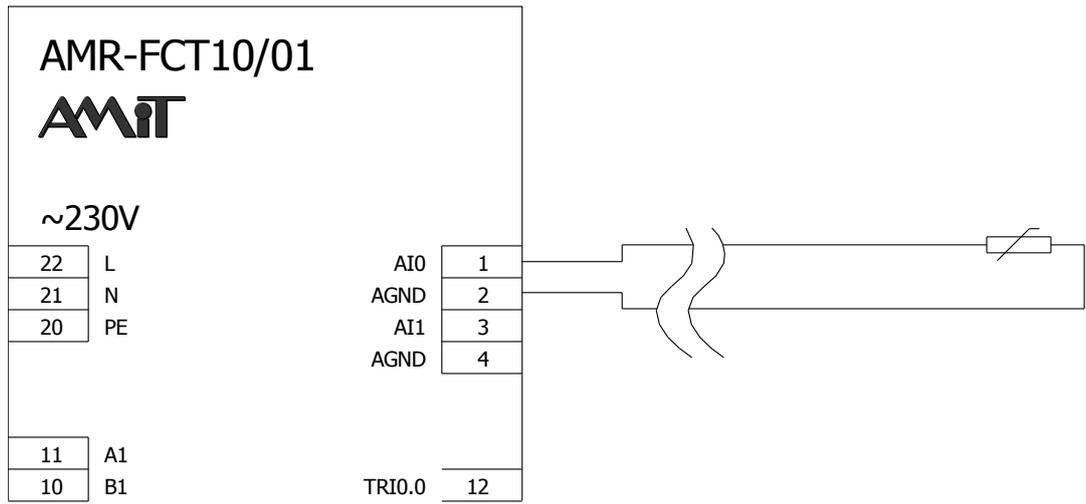
Fig. 11 – Temperature sensor wiring example
