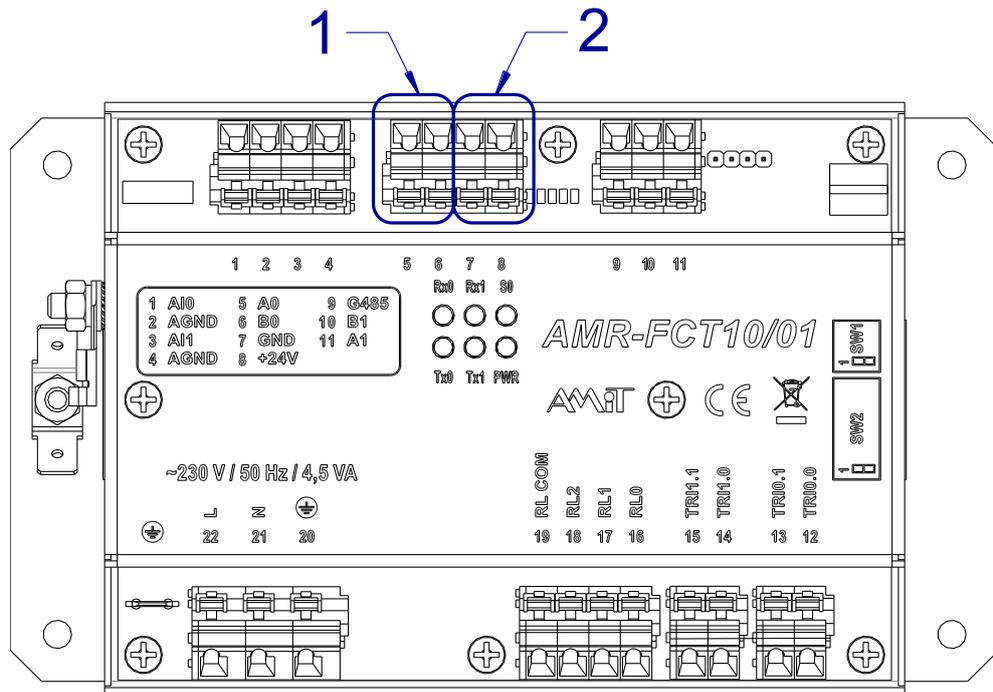
Fig. 6 – Terminals location for on-wall controller connection
