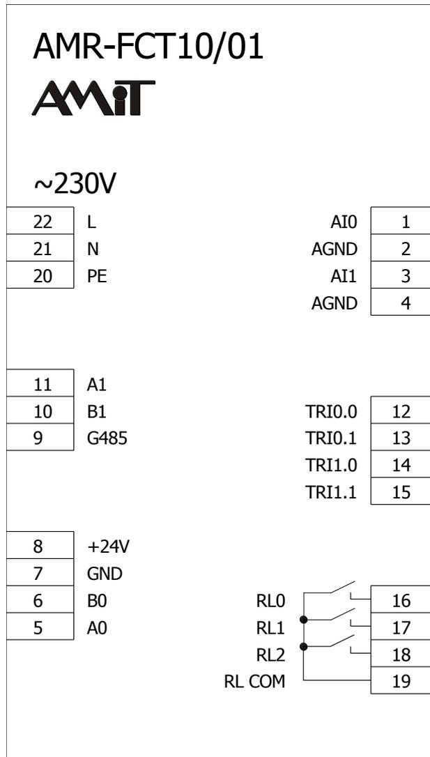
Fig. 2 – Recommended drawing symbol for **AMR-FCT10/01**
