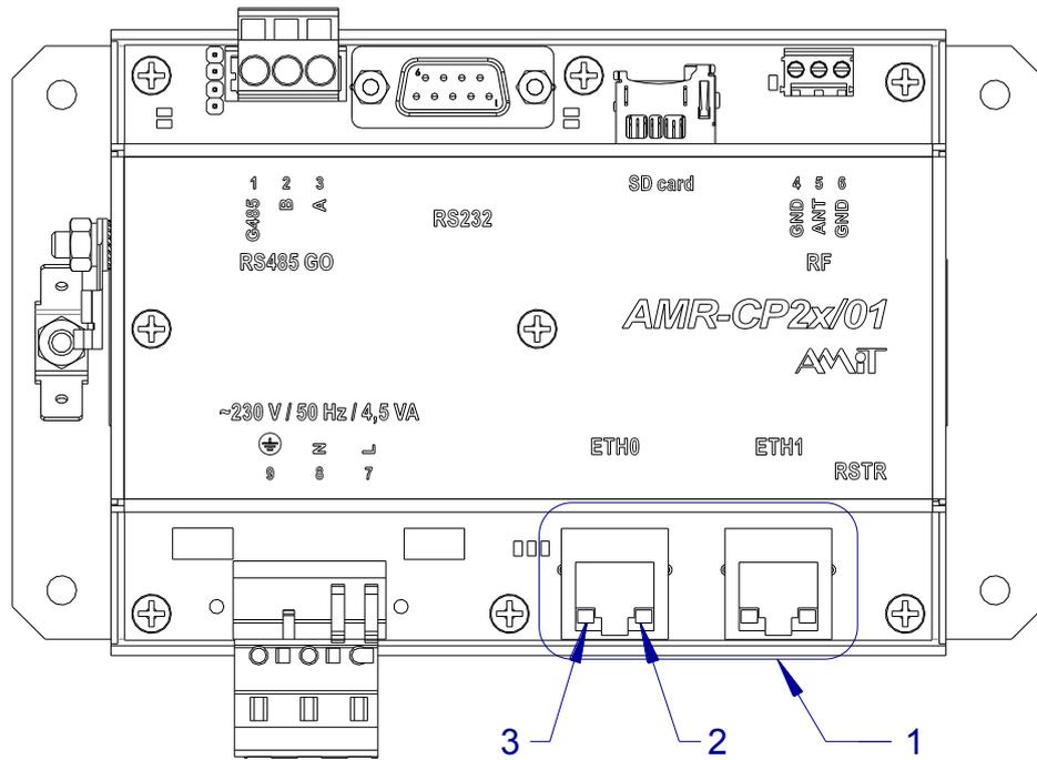
Fig. 7 - Ethernet ETH0 and ETH1 connector location
