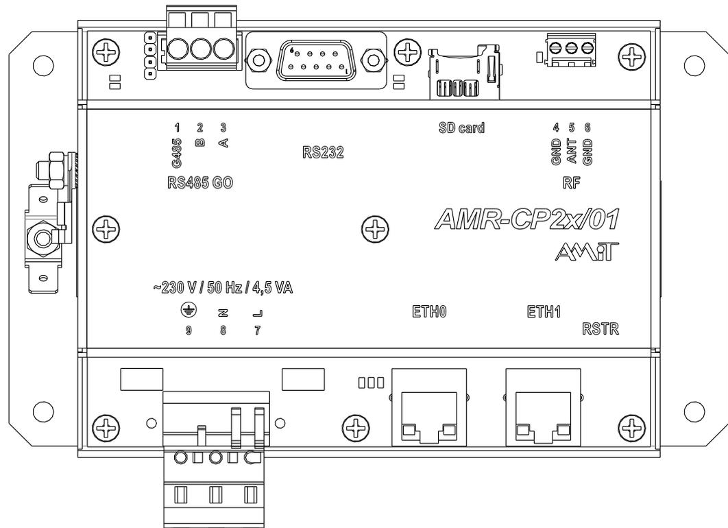
Fig. 10 - Connectors and terminals layout
