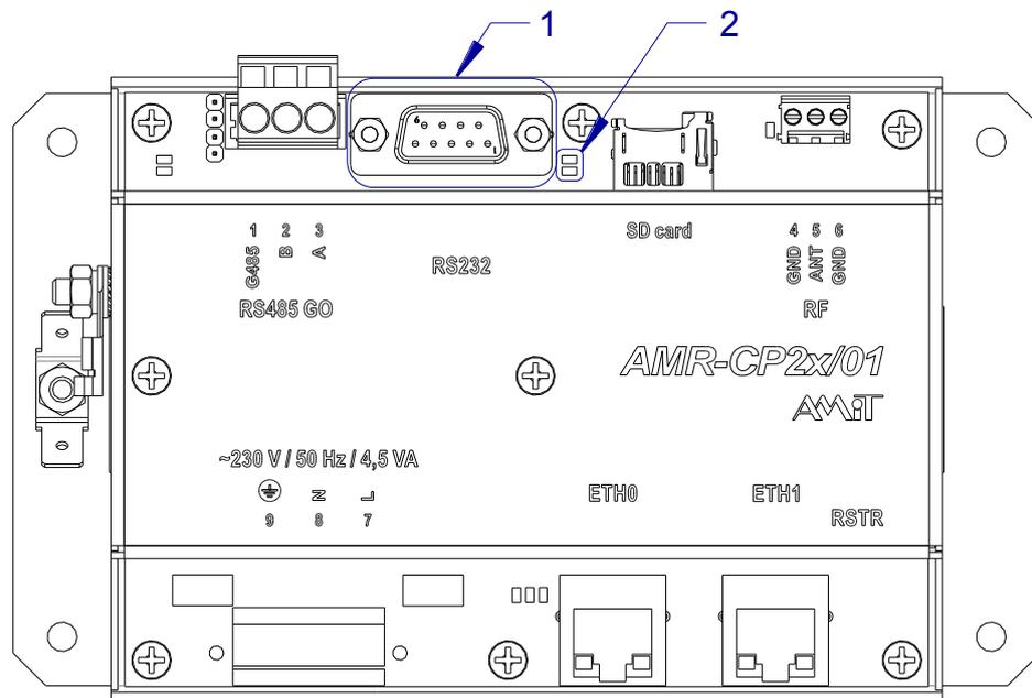
Fig. 5 - RS232 connector location
