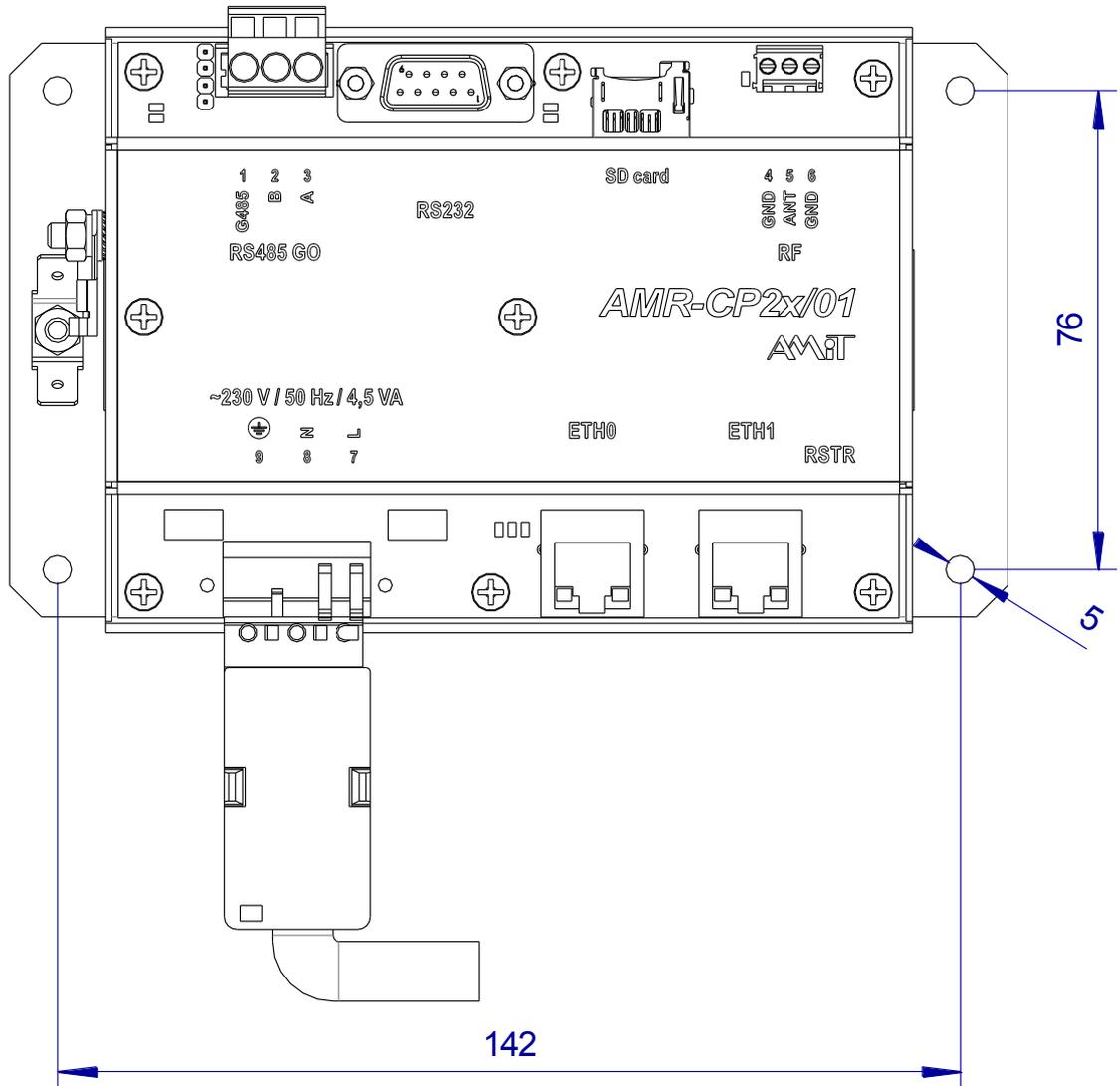
Fig. 11 - Dimensions of mounting holes
