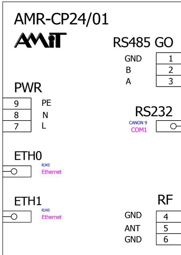
Fig. 2 - Recommended drawing symbol for **AMR-CP24/01**
