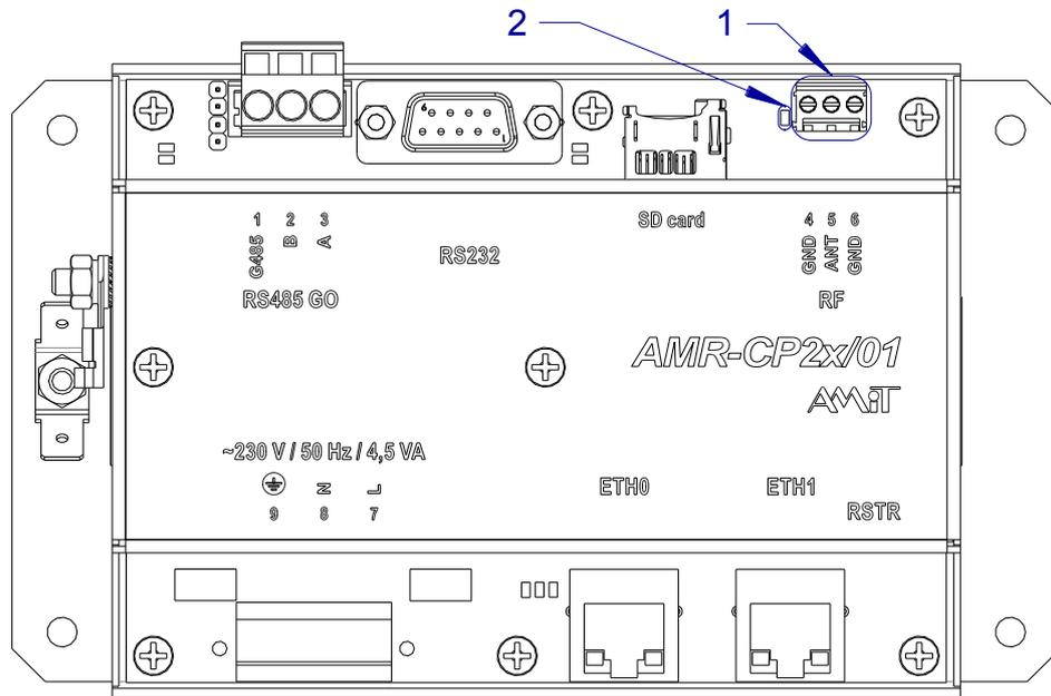
Fig. 8 - Location of the Poseidon system antenna connector
