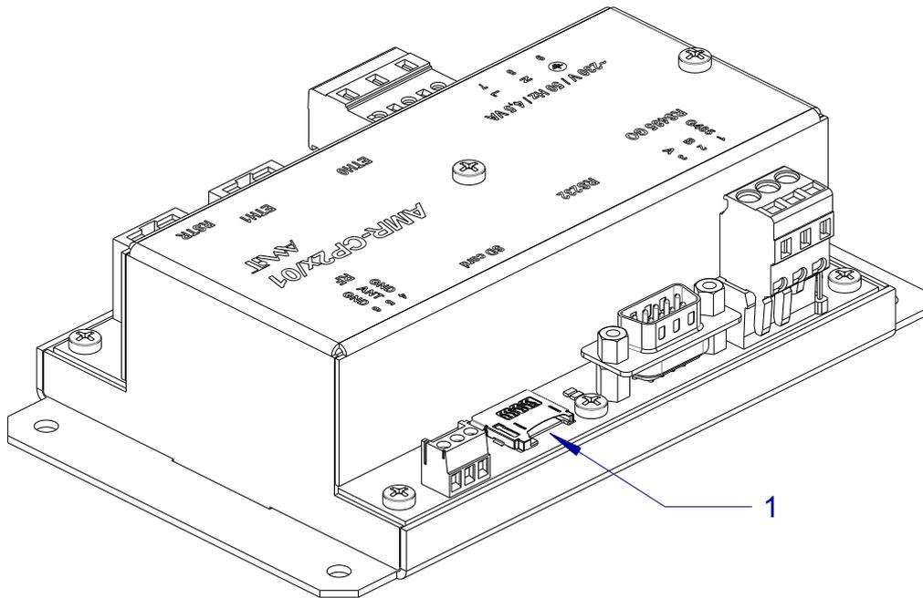
Fig. 9 - Location of Micro SD card slot
