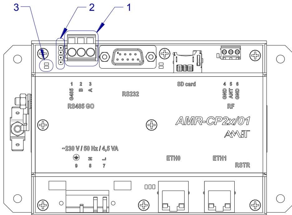
Fig. 6 - RS485 connector location
