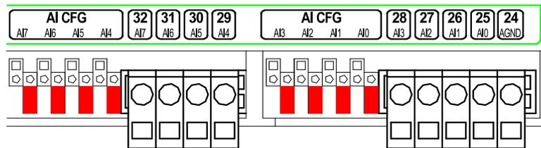
Fig. 15 - Setting configuration jumpers for 0 V to 10 V range, digital input 24 V
