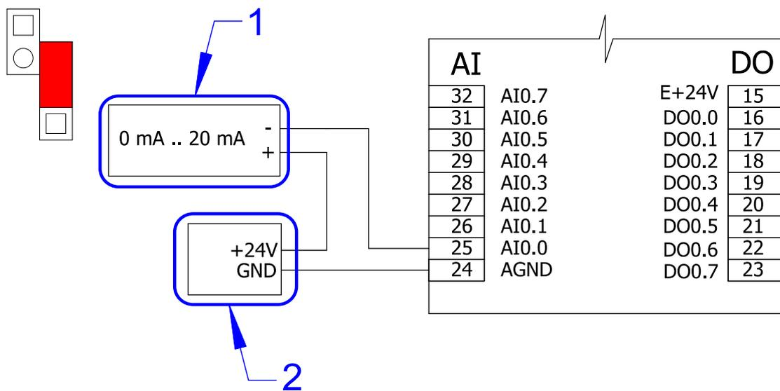
Fig. 21 - Connecting sensor with current output 0 mA to 20 mA (4 mA to 20 mA)
