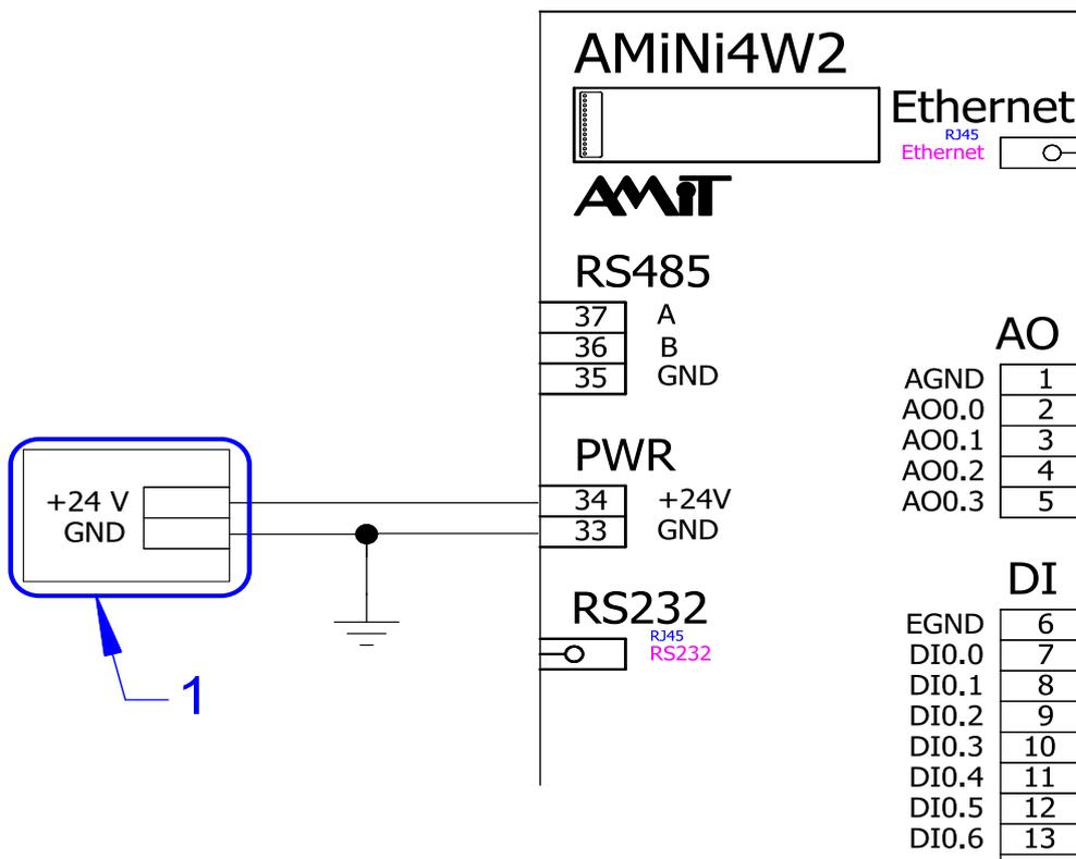
Fig. 4 - Wiring example of single control system
