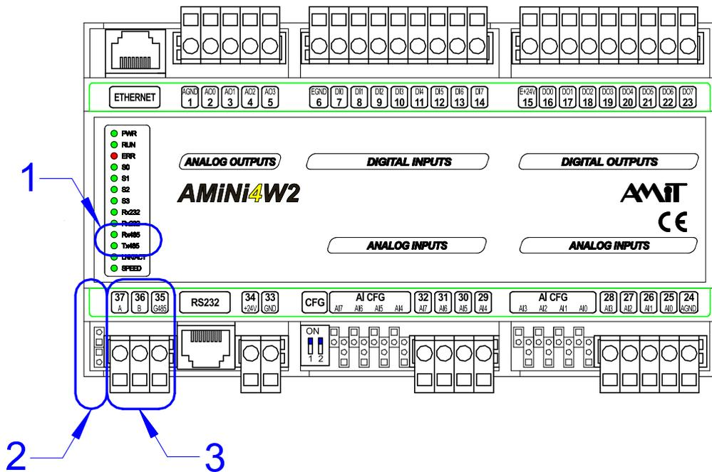
Fig. 28 - RS485 connector and indication LEDs location
