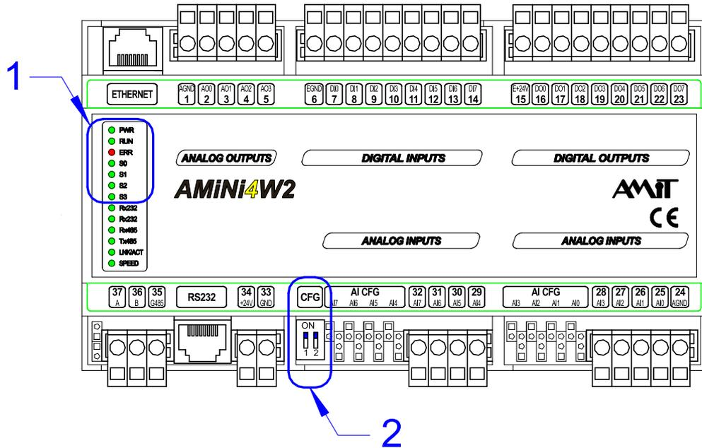
Fig. 33 - DIP switch and status indicator locations
