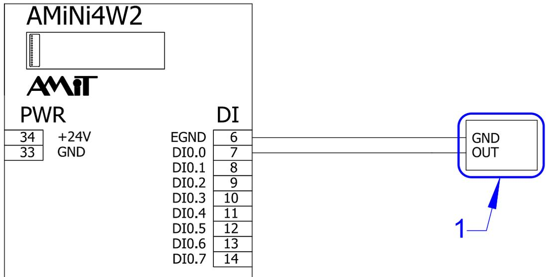
Fig. 8 - Connecting self-supplied active output
