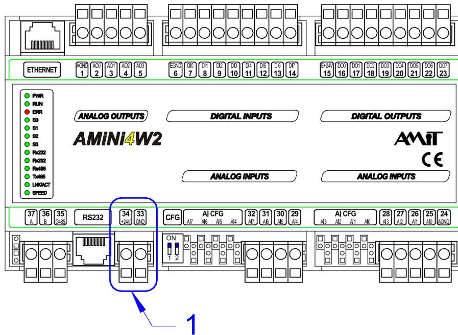
Fig. 3 - Power supply connector location
