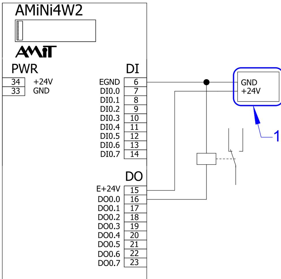
Fig. 11 - Operating the power contactor by semiconductor output
