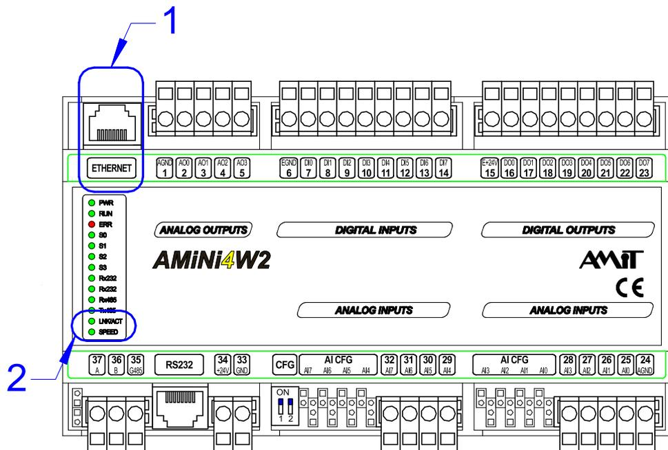
Fig. 31 - Ethernet connector and indication LEDs location
