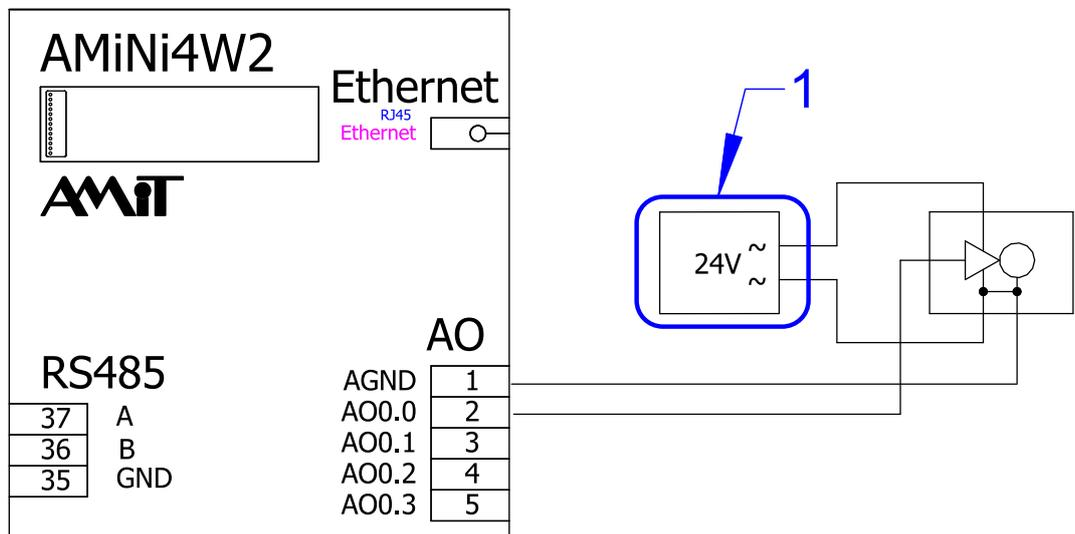
Fig. 25 - Connecting AC supplied servo
