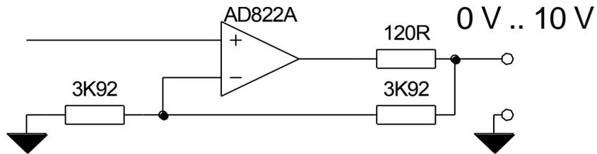
Fig. 24 - Wiring scheme of final stage of single channel analogue output
