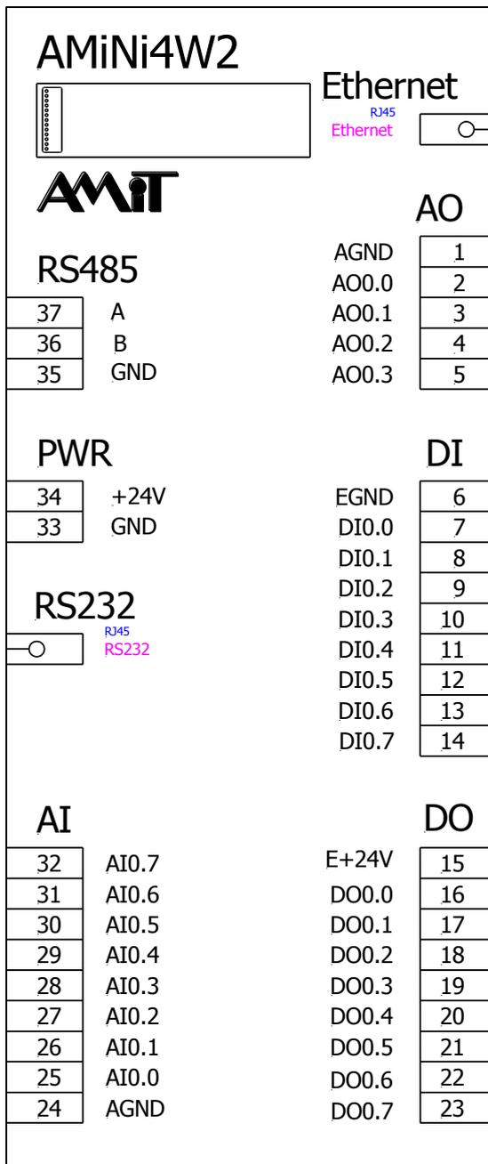
Fig. 2 - Recommended drawing symbol for **AMiNi4W2**
