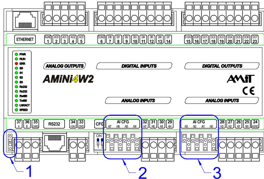
Fig. 34 - Configuration jumpers location
