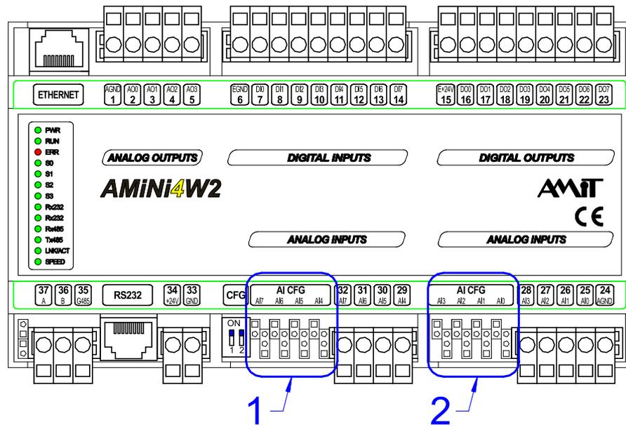
Fig. 18 - Configuration jumpers location
