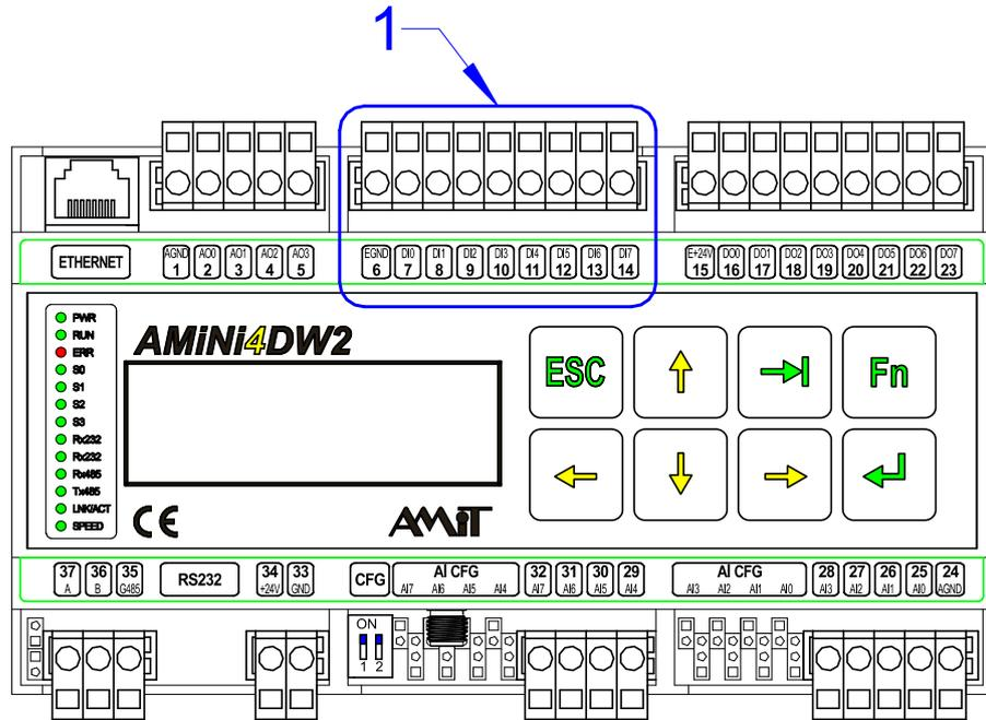
Fig. 5 - Inputs DI0.0 to DI0.7 connector location
