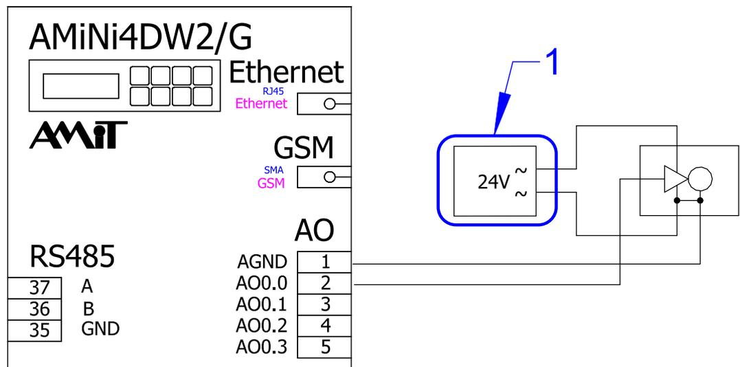
Fig. 25 - Connecting AC supplied servo
