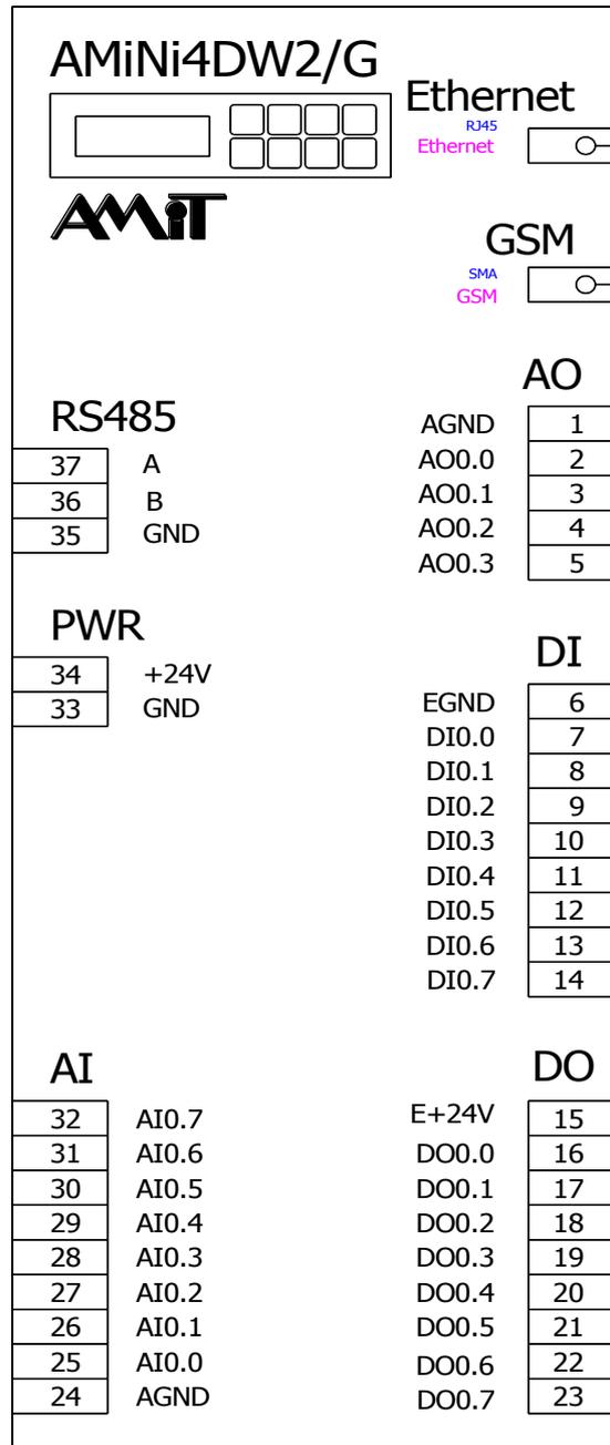
Fig. 2 - Recommended drawing symbol for **AMiNi4DW2/G**
