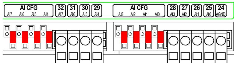
Fig. 16 - Setting configuration jumpers for 0 mA to 20 mA range
