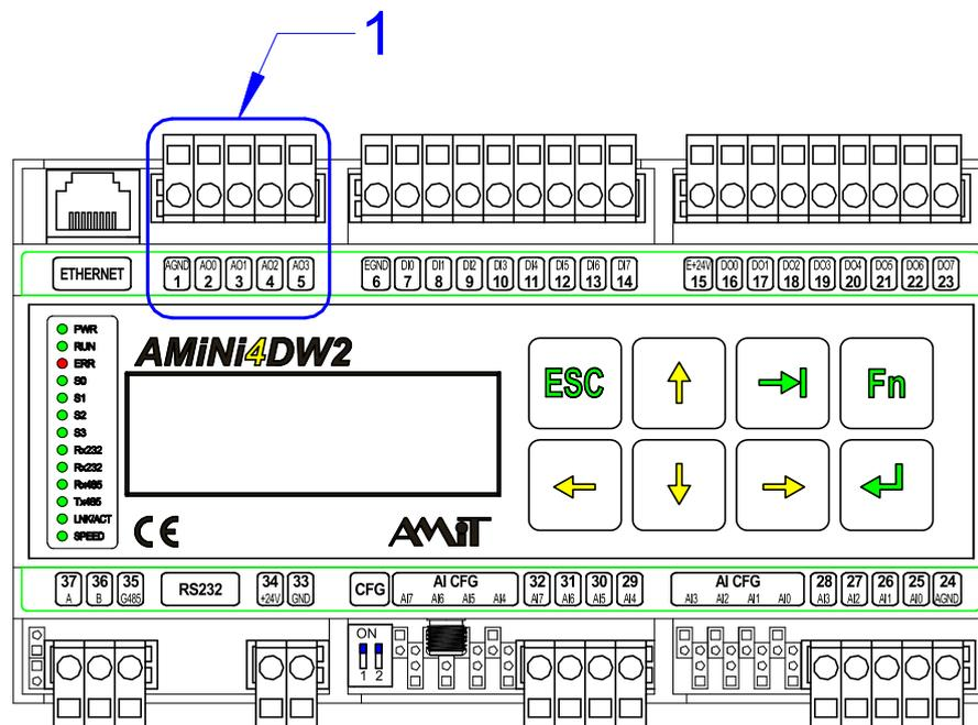
Fig. 23 - Outputs AO0.0 to AO0.3 connector location
