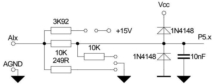
Fig. 13 - Wiring scheme of analogue input single channel
