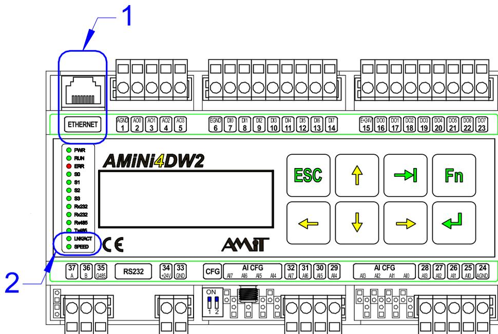
Fig. 29 - Ethernet connector and indication LEDs location
