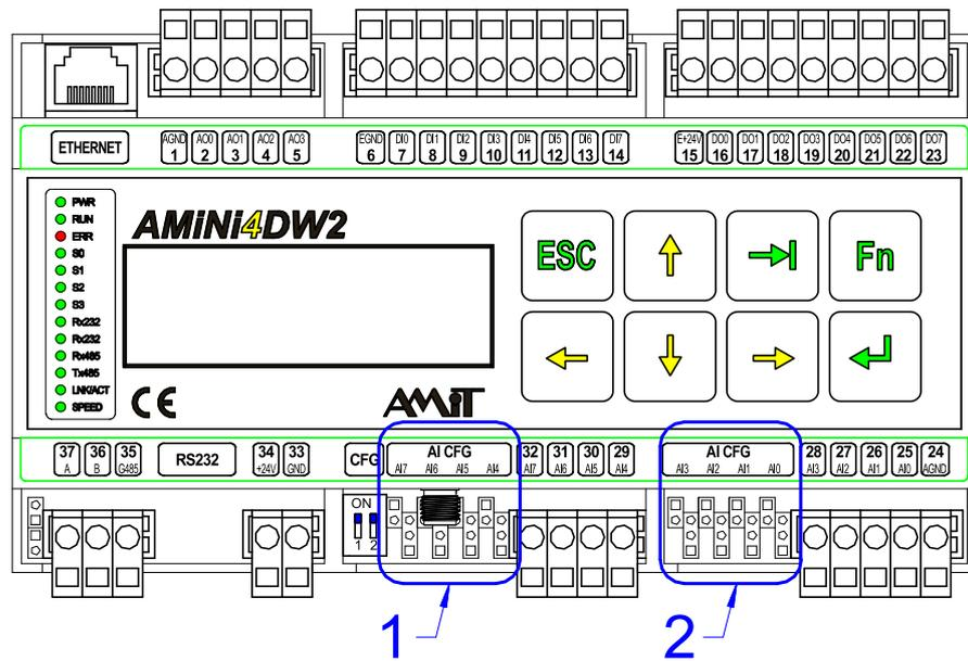
Fig. 18 - Configuration jumpers location
