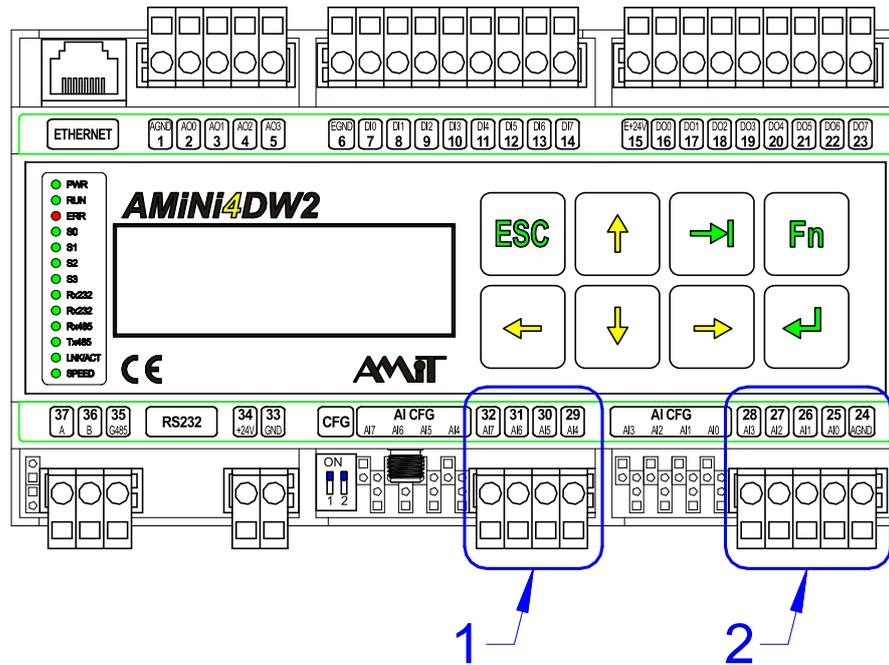
Fig. 12 - Inputs AI0.0 to AI0.7 connectors location
