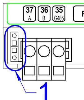
Fig. 28 - Disconnected jumpers on end station
