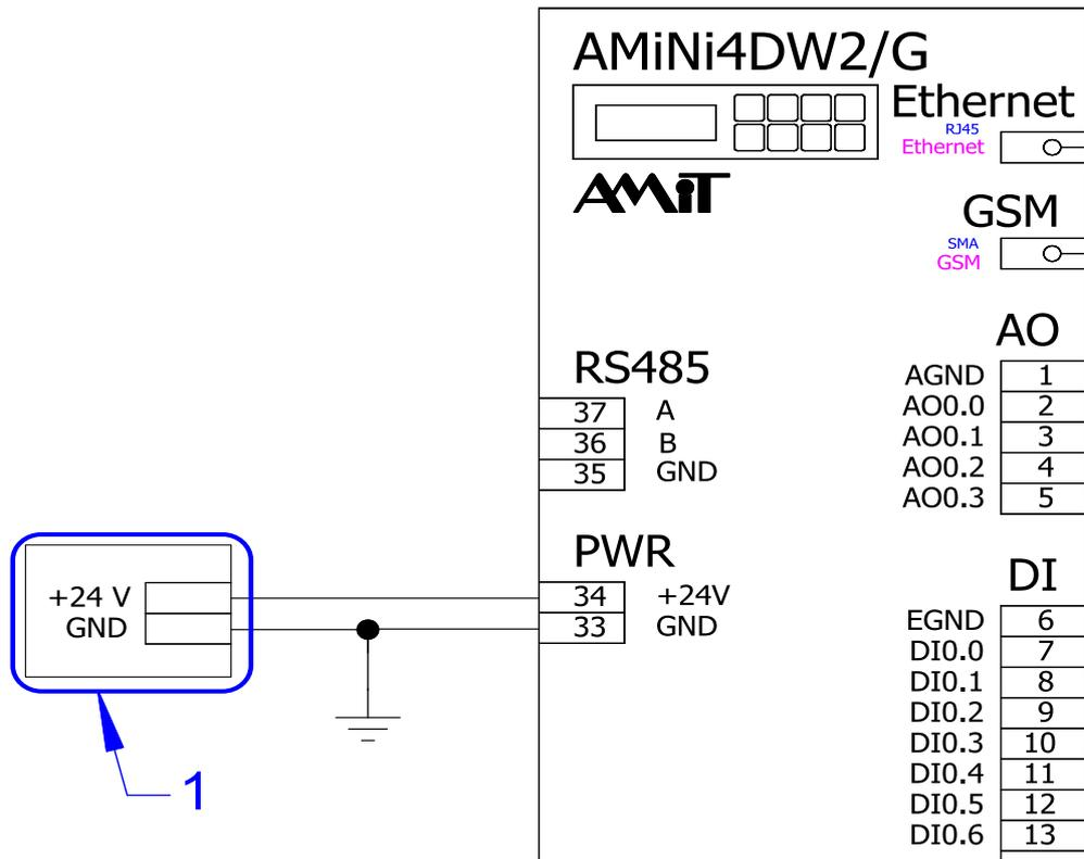
Fig. 4 - Wiring example of single control system
