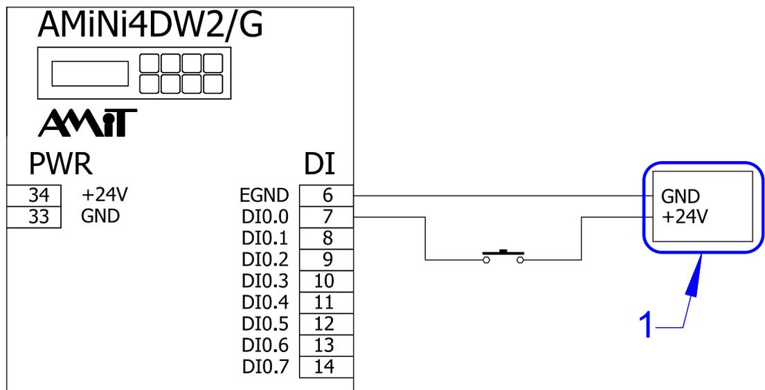
Fig. 7 - Passive contact supplied from individual power supply
