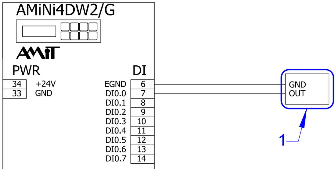
Fig. 8 - Connecting self-supplied active output
