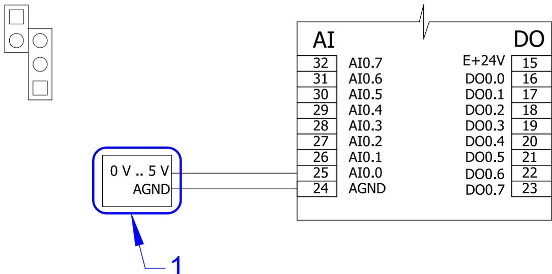
Fig. 19 - Connecting voltage sensor 0 V to 5 V
