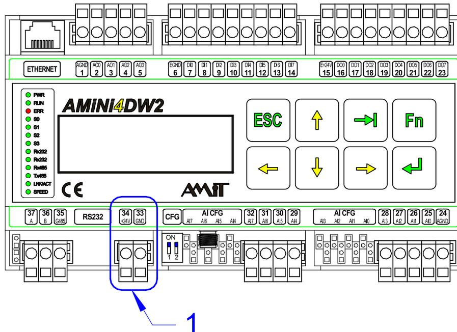
Fig. 3 - Power supply connector location
