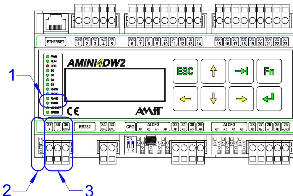
Fig. 26 - RS485 connector and indication LEDs location
