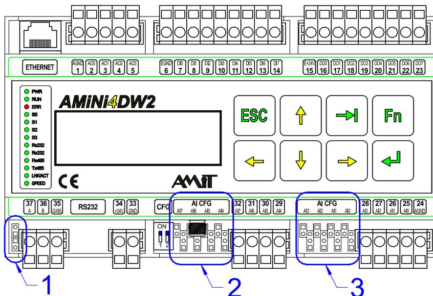
Fig. 34 - Configuration jumpers location
