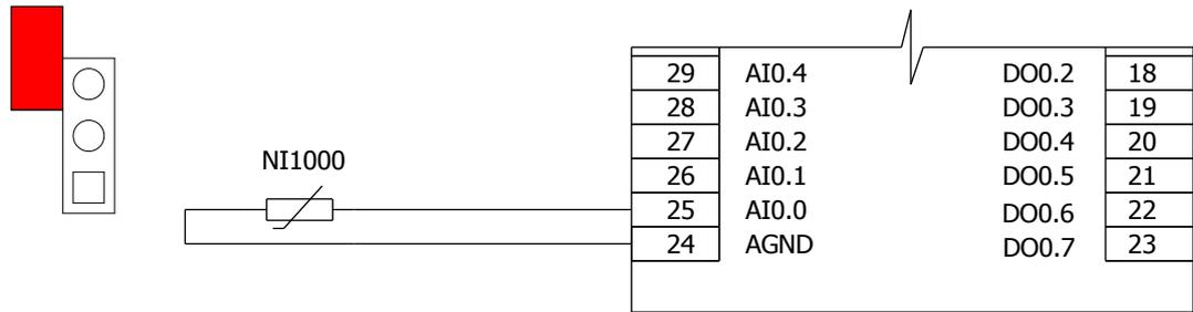
Fig. 22 - Connecting Ni1000 sensor
