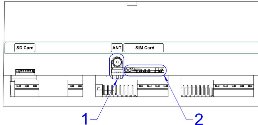
Fig. 30 - Antenna connector and slot for SIM card location
