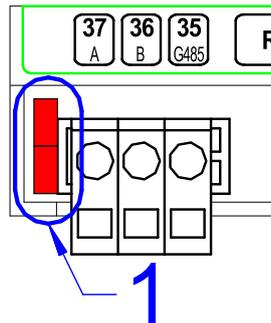
Fig. 27 - Connected jumpers on end station
