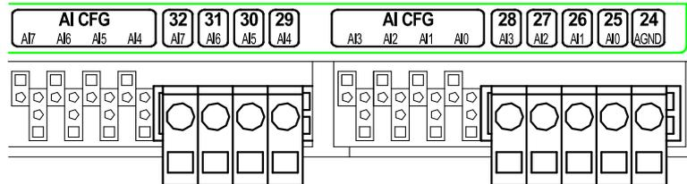
Fig. 14 - Setting configuration jumpers for range 0 V to 5 V
