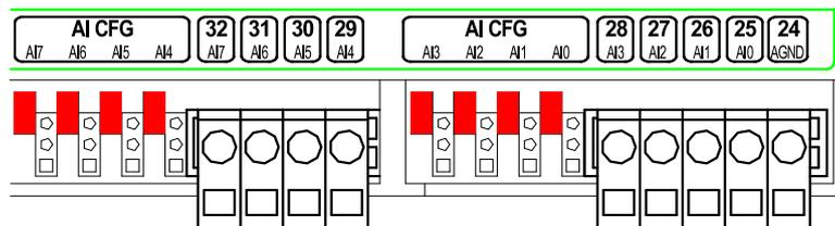
Fig. 17 - Setting configuration jumpers for Ni1000 / Pt1000 sensors
