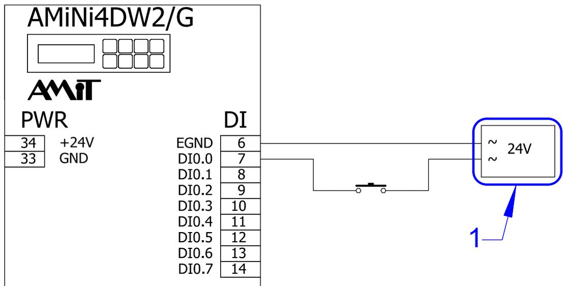
Fig. 9 - Passive contact supplied from AC power supply
