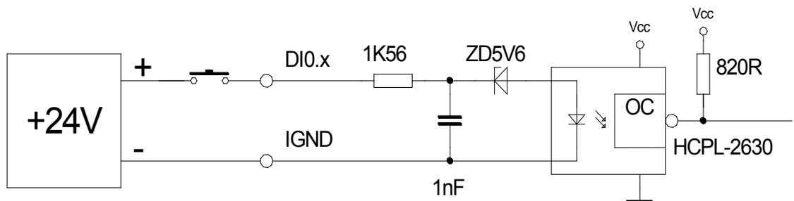
Fig. 6 - Wiring scheme of single digital input channel
